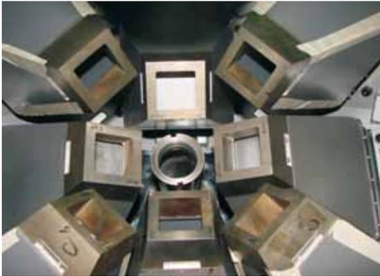
Fig. 3. Beam tube surrounded by anti-Compton shields
