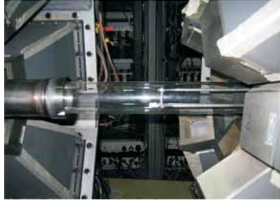
Fig. 4. Cylindrical scattering chamber with target mounted
