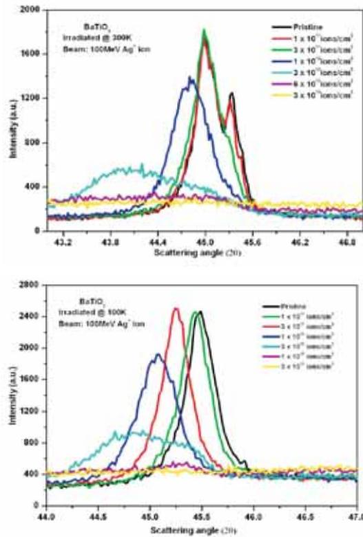
**Fig.1.** In-situ X-ray diffractometer spectra of pristine and irradiated (BaTiO<sub>3</sub> samples) with <sup>108</sup>Ag<sup>+9</sup> ions at (a) 300K and (b) 100K with ion fluence varying from 1x10<sup>11</sup> to 3x10<sup>13</sup> ions/cm<sup>2</sup>
