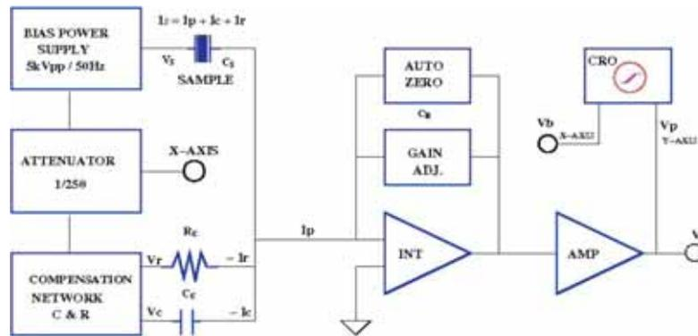
Fig.1. Block diagram of electric field (E) versus polarization (P) measurement setup
