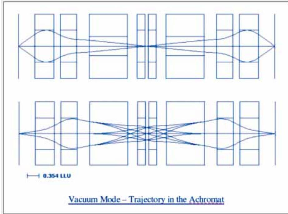
Fig. 2. Trajectories of particles in momentum achromat mode of HYRA (first stage)
