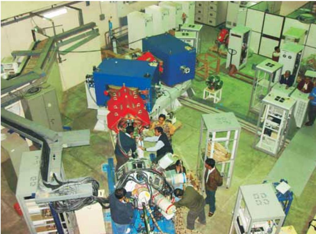
**Fig. 2. INGA Array with HYRA during installation phase**
