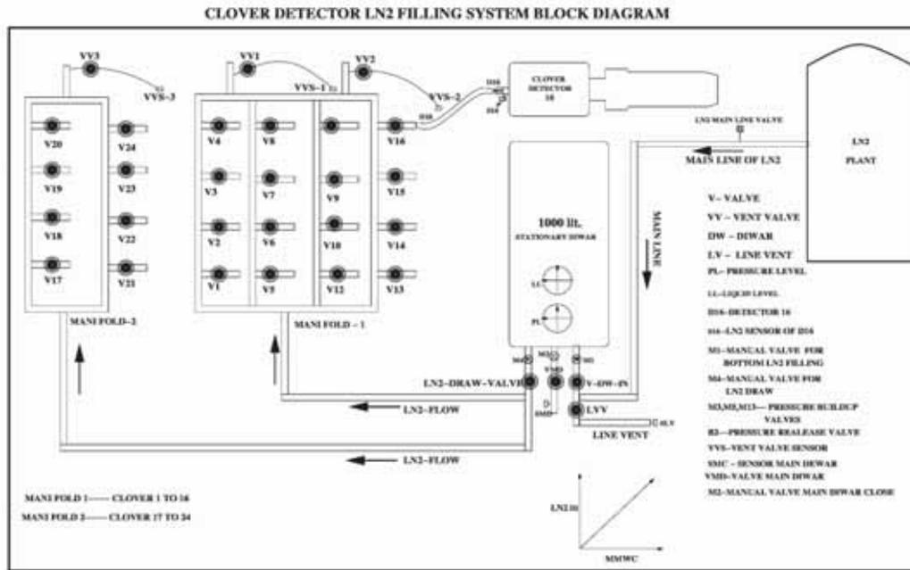
Fig. 6. Schematic diagram for LN2 Autofill system of INGA
