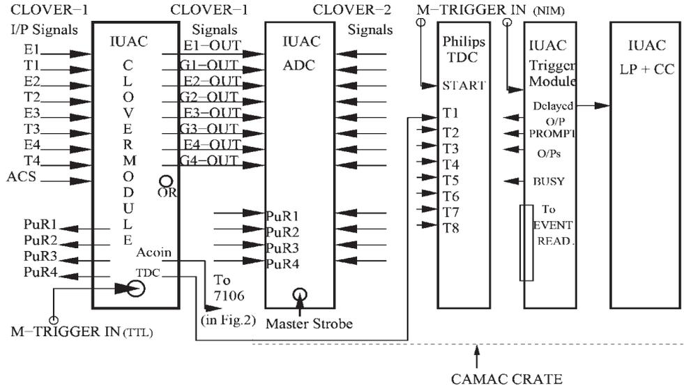
**Fig. 8. Schematic diagram for Event trigger of INGA**
