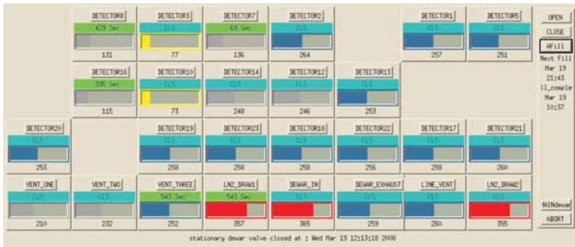
Fig. 7. Graphical User Interface for Autofill System
