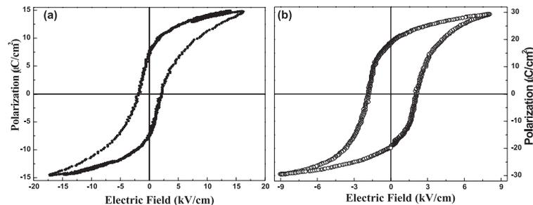
Fig.2. Hysteresis loop at room temperature for (a) BaTiO<sub>3</sub> and (b) (PbNi<sub>1/3</sub>Nb<sub>2/3</sub>-PbZr<sub>0.34</sub>Ti<sub>0.66</sub>)O<sub>3</sub>
