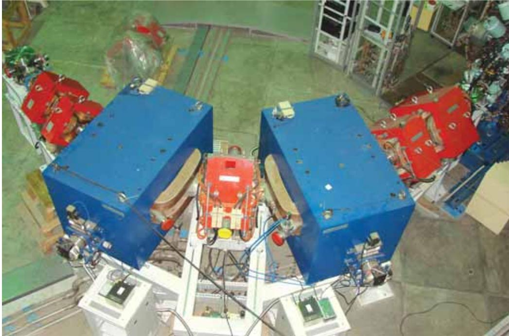
**Fig. 1. HYRA first stage momentum achromat coupled with INGA facility**
