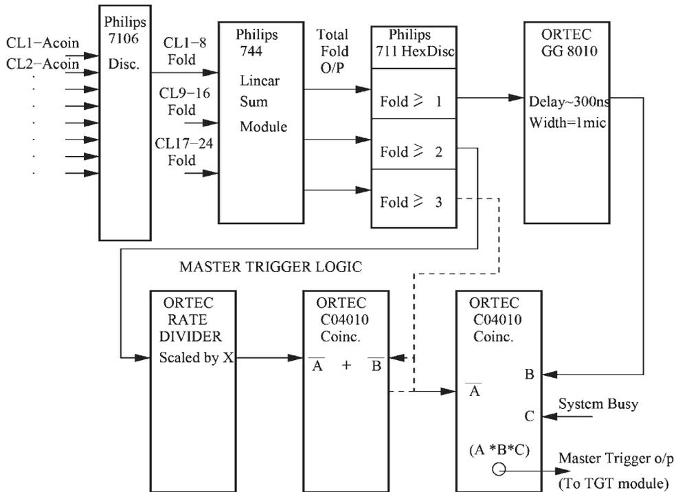
**Fig. 9. Schematic diagram Data Acquisition of INGA**
