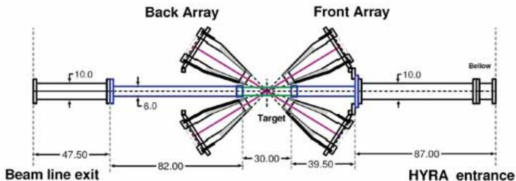
Fig. 5. Schematic layout of the beam line for INGA (all dimensions in cm units)
