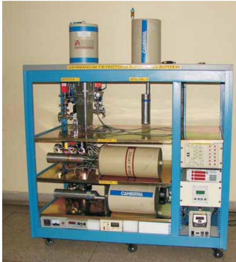
**Fig 12. Annealing station for Ge detectors**
