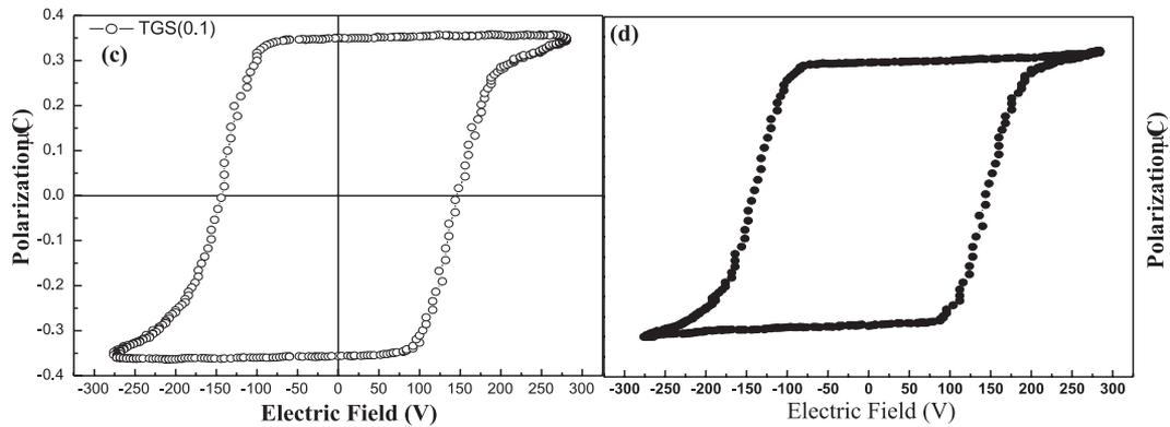
**Fig.3. Hysteresis loop of TGS single crystal for (c) Uncompensated and (d) Compensated one**
