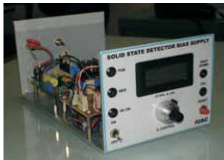
Fig. 7. 1kV/20uA Surface barrier detector bias supply
