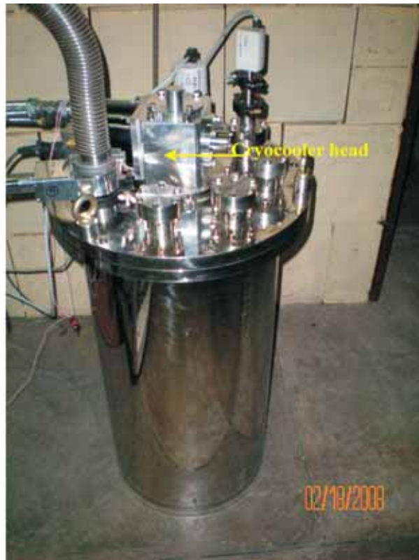
Fig. 8. Cryocooler test set up
