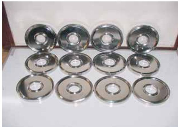
Fig. 1. Niobium Top Flanges after electropolishing. Twelve, out of the fifteen, flanges are shown
