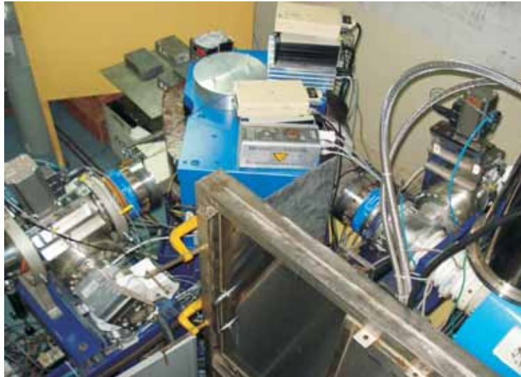
Fig. 1. PKDELIS ECR source and low energy beam transport
