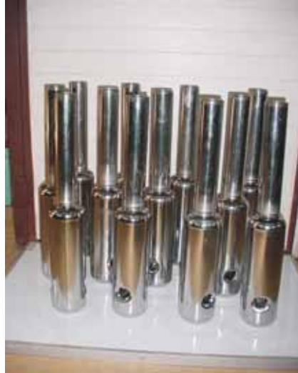
Fig. 2. Niobium Central Conductor assemblies. Twelve, out of the fifteen, assemblies are shown
