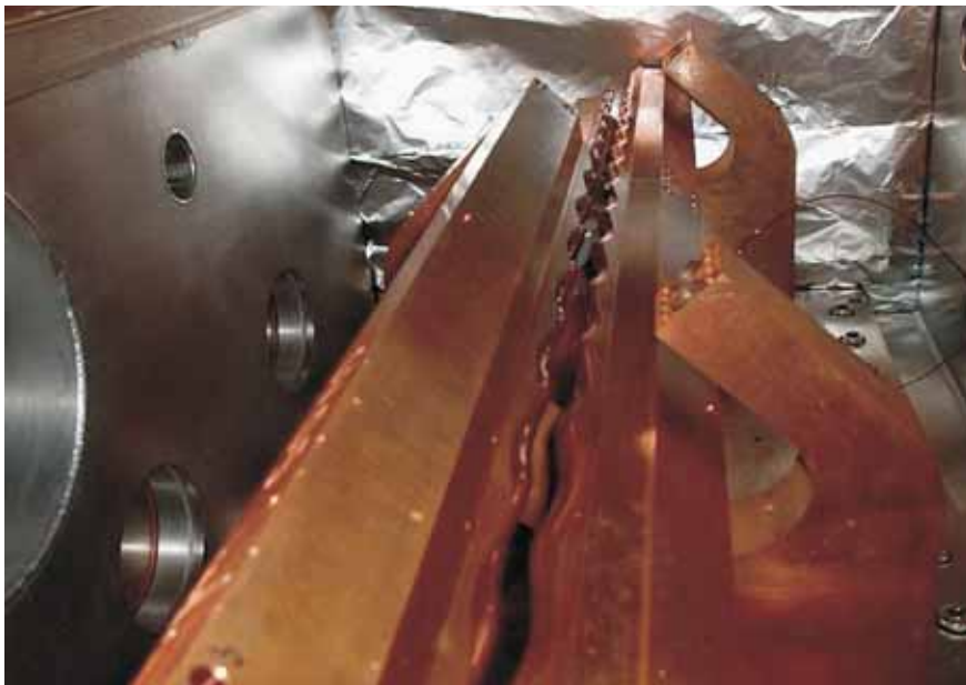
Fig.1. General Assembly of the 1.17m modulated RFQ at IUAC
