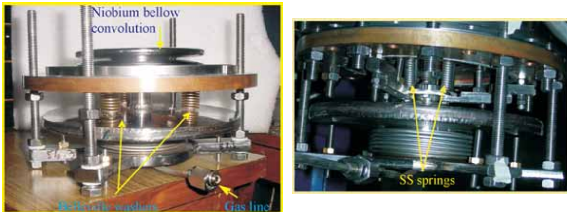
Fig. 3. The first picture shows the slow tuner fixture with Belleville washers (old design). The second picture shows the washers are replaced by SS-springs (new design)
