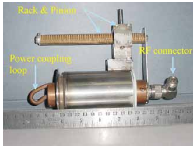
Fig. 2. The new drive coupler which is now installed in all the resonators in SB, linac and RB cryostats
