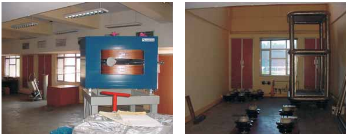
Fig. 3. Left: New switcher magnet ; Right: 300 kV high voltage platform
