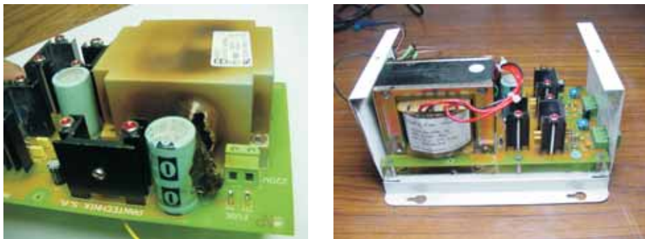
Fig. 1. (a): (Left) PCB of gas controller valve (before repair); (b): (Right) PCB of gas controller valve (after repair)
