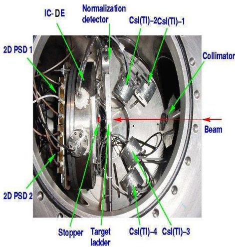
**Fig. 1: Experimental setup for measuring elastic/transfer & fusion for  ${}^7\text{Be} + {}^{27}\text{Al}$  system**
