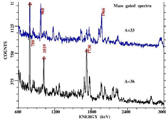
**Fig. 1: Recoil gated  $\gamma$ -spectra with gates on A=33 and A=36 respectively**
