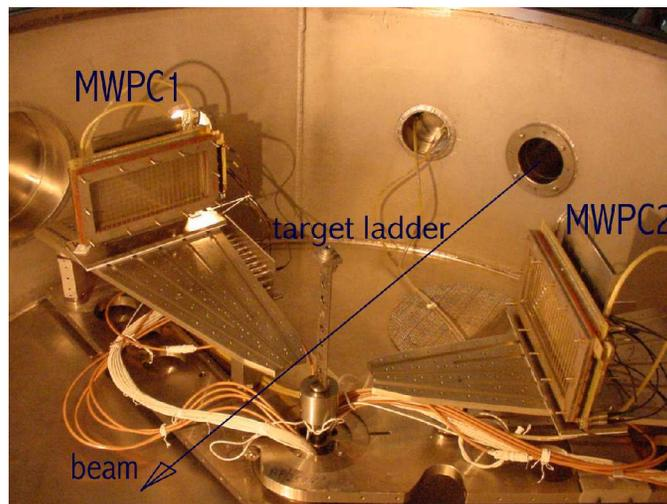
**Fig. 1: Detectors placed inside GPSC**
