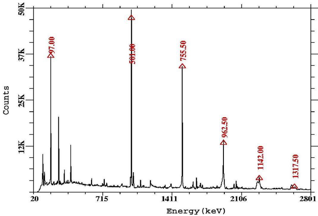
Fig. 2 : The added gated spectra of 97+ 501+756+963 +1142 keV peaks in  $^{79}\text{Rb}$
