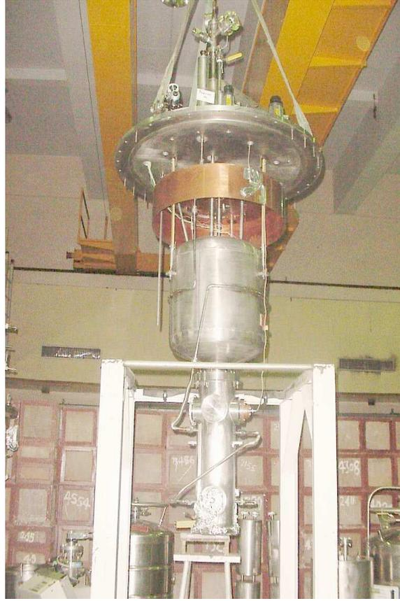
**Fig. 11 : Simple Test Cryostat top insert with a resonator**
