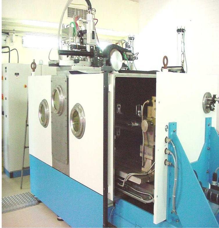
**Fig. 3 : Electron Beam Welding Machine at Nuclear Science Centre**
