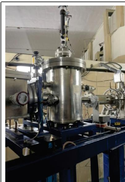
Fig. 1- Proton ion beam chamber
