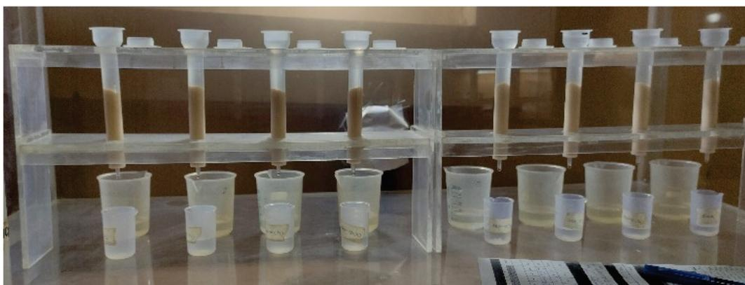
Fig.1 (C) Cation column separation of samples
