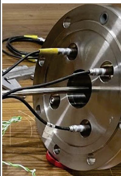
Fig. 2- Cable connections to feedthrough
