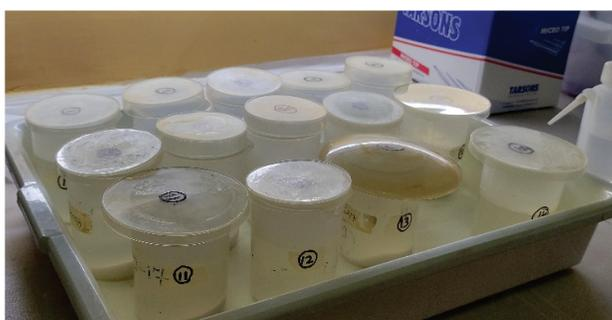
Fig.1 (a) Samples ready for acid digestion
