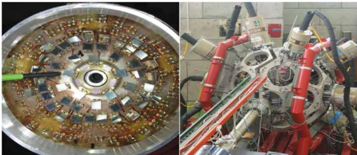
Fig 6. (a) The backward hemisphere of the Munich chamber equipped with 48 PIN diodes of  $0.5 \times 0.5 \text{ cm}^2$  active area for the detection of back-scattered beam and (b) EAGLE array consisting of 15 HPGe detectors equipped with anti-Compton BGO shields.
