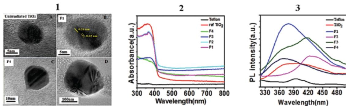
Fig. 1. TEM micrograph of un-irradiated A) and irradiated TiO<sub>2</sub> nanoparticles with fluences of B) F1 and C) F4. The formation of ripples is shown in D). Fig. 2. UV-Vis optical absorption spectra and Fig. 3. PL spectra of irradiated and un-irradiated particles.
