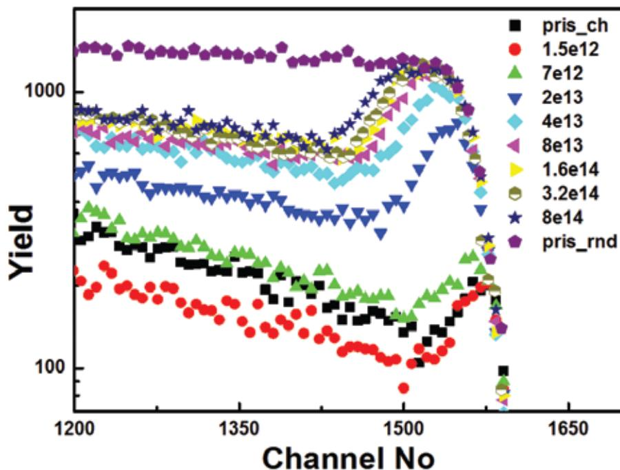
Fig. 1 Channeled spectra of irradiated and pristine Ge samples
