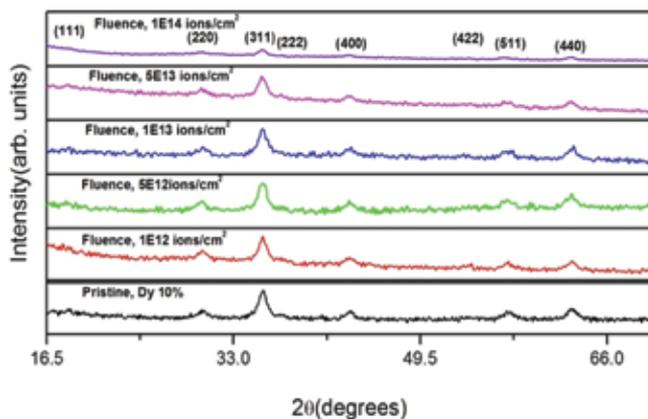
Fig. 1. XRD pattern of pristine and irradiated sample of  $\text{CoFe}_{1.90}\text{Dy}_{0.10}\text{O}_4$ .
