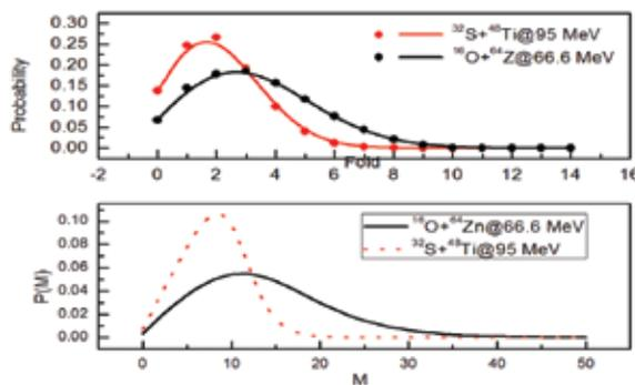
Fig. 3. Comparison of fitted fold distributions (top) and extracted gamma multiplicity distributions (bottom) for both the systems at  $E^* = 52.8$  MeV.
