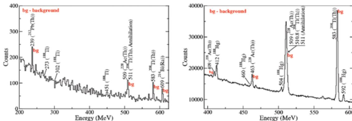
Fig 3: Addback spectrum in focal plane Clover detector with (right) and without (left) gate on ERs identified by the MWPC and Si pad detectors.
