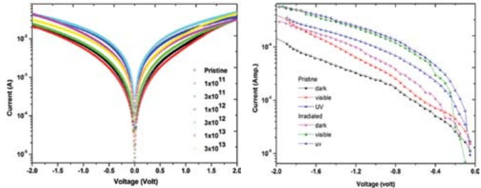
Fig. 2 (a) *In-situ* current-voltage (I-V) characteristics of ZnS:TiO<sub>2</sub>/p-Si QD's heterojunction at different SHI fluences (b) current-voltage characteristics under the visible and UV light of the pristine and irradiated ZnS:TiO<sub>2</sub>/p-Si QDs heterojunction photo diode
