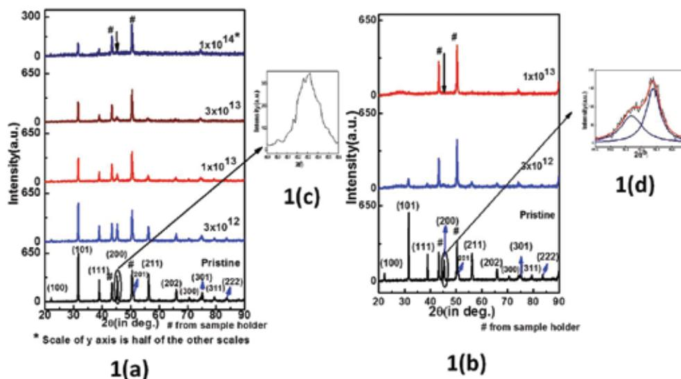
Fig.1 (a) and Fig.1(b) shows XRD patterns of BaTiO<sub>3</sub> before and after irradiation with 100-MeV Ag ions at different fluences at 25 K and 300 K respectively and Fig. 1(c) and Fig.1 (d) shows effect of temperature change on shape of diffraction peak around angle  $45^\circ$ .
