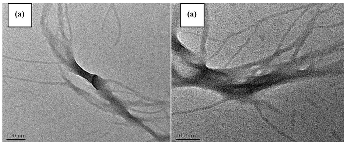
Fig. 1. HRTEM micrographs of (a) pristine and (b) irradiated PAni nanofibers at fluence 3×10<sup>11</sup> ions/cm<sup>2</sup>.
