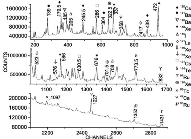
Fig. 1. Gated  $\gamma$ -ray spectra obtained from  $^{32}\text{S} + ^{92}\text{Mo}$  reaction.
