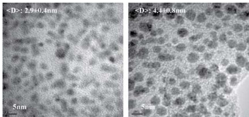
Fig.1. TEM images of as-deposited (left), and SHI ion irradiated (right) the Pd NPs embedded in silica matrix.
