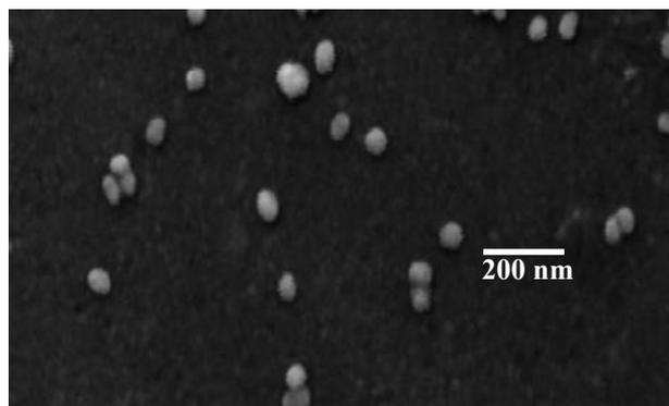
Fig. 2. Scanning Electron Microscopy (SEM) of AuNP.
