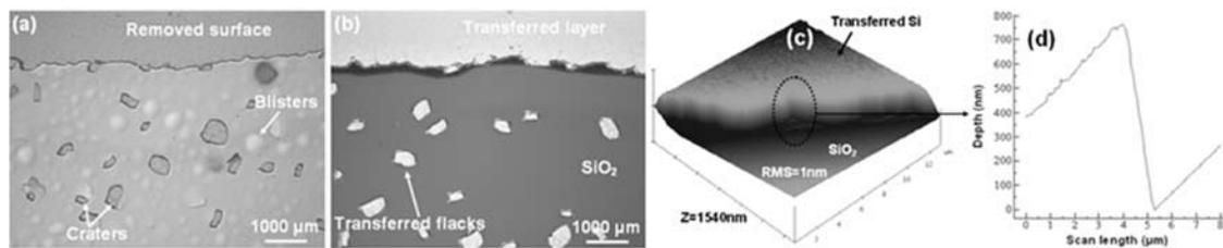
Fig. 1. Nomarski optical images of the surfaces of Si wafers after debonding/splitting following the annealing steps; (a) H-implanted Si wafer and (b) oxidized Si wafer. (c) Shows the AFM image of the transferred Si layer and (d) represents its thickness.
