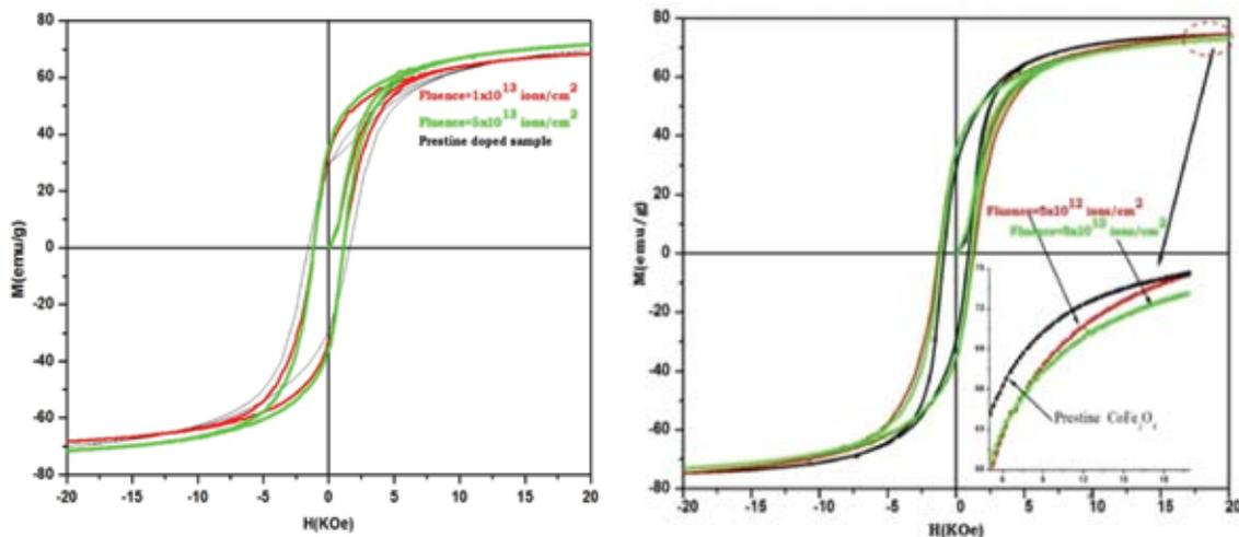
Fig. 1. M-H curves for (left) pristine and (right) irradiated cobalt ferrite at different fluencies.
