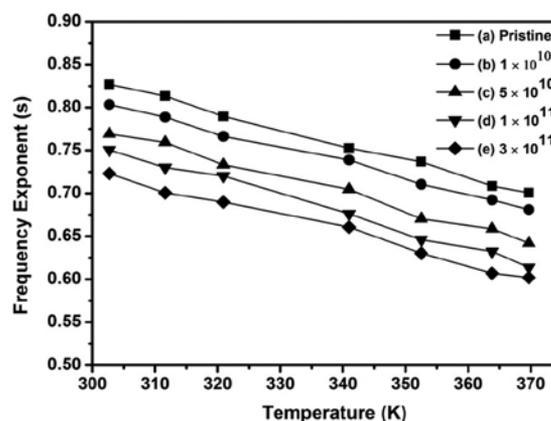
Fig. 3. Temperature dependent of frequency exponent  $s$  of the pristine and irradiated PANi nanofibers at fluence  $10^{10}$ ,  $5 \times 10^{10}$ ,  $10^{11}$  and  $3 \times 10^{11}$  ions/cm<sup>2</sup>.
