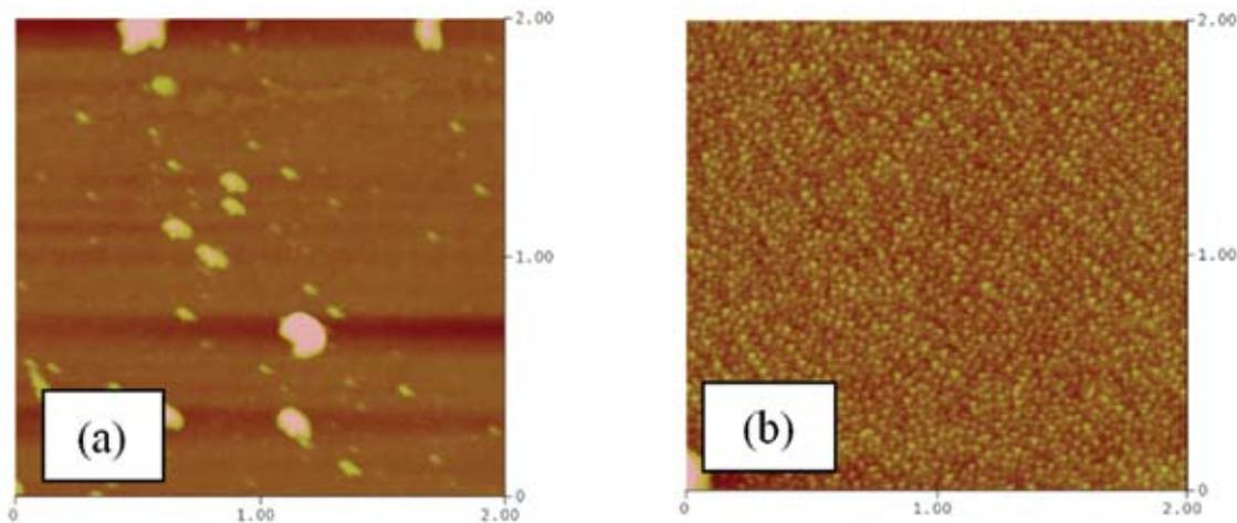
Fig. 1 AFM images of (a) pristine and (b)  $1 \times 10^{12}$  ions/cm<sup>2</sup> irradiated samples. The scan size is 2  $\mu$ m. The initially random pristine surface structure has been transformed into an array of well-developed nanostructures of fairly uniform lateral size of 30-40 nm due to 100 MeV O ion irradiation.
