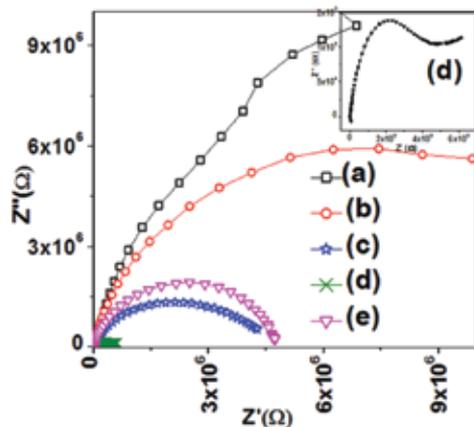
Fig. 1. Impedance Cole-Cole Plot for (a) unirradiated and irradiated blends at fluences of (b)  $1 \times 10^{11}$ , (c)  $3 \times 10^{11}$ , (d)  $1 \times 10^{12}$  and (e)  $3 \times 10^{12}$  ions/cm<sup>2</sup>.
