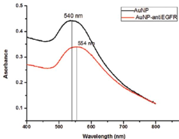
Fig. 3. UV-Vis absorbance of Au nanoparticles and Au nanoparticle conjugated with anti EGFR.
