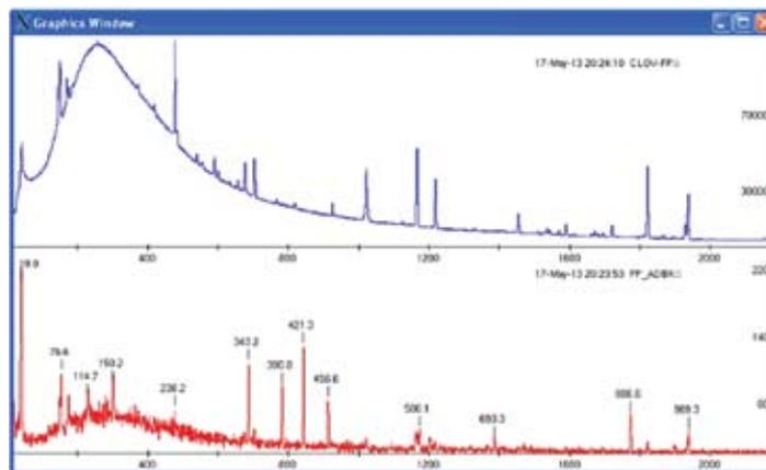
Fig. 2. Add-back spectrum in focal plane Clover detector with (bottom) and without (top) gate on ERs, identified by MWPC and Si pad detectors. The marked peaks are mostly from isomeric decay in  $^{195}\text{Bi}$ .
