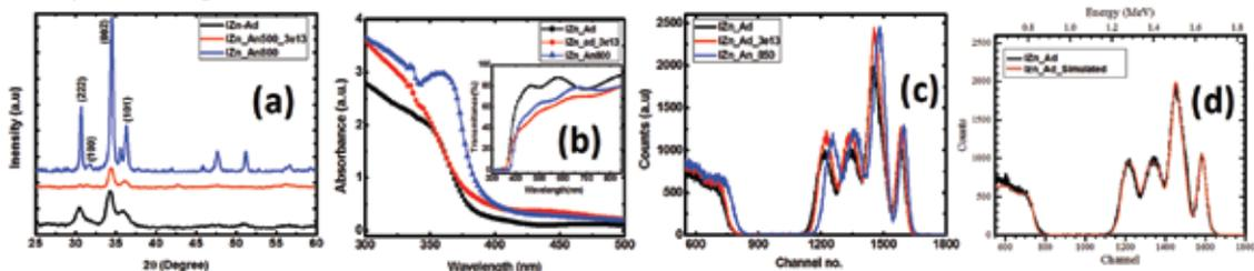
Fig. 1 (a) GIXRD pattern, (b) Absorption and transmission spectra (c) RBS spectra of as-deposited, irradiated and thermally annealed  $ZnO/In/ZnO/In/ZnO$  on silicon and/or silica substrate, (d) experimental and simulated RBS spectra of as-deposited sample on silicon substrate.
