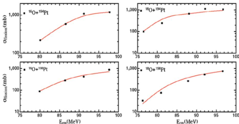
Fig. 2 : Experimental fission cross section for  $^{16,18}\text{O} + ^{194,198}\text{Pt}$  reactions. Red lines are the calculated values from PACE2 code.
