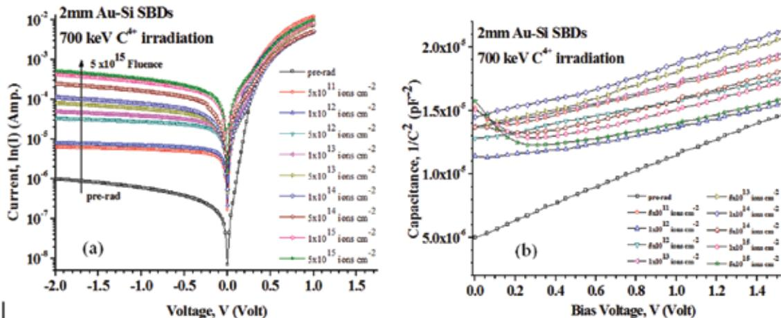
Fig. 1. (a) I-V characteristics of Au/n-Si (100) SB diodes at different ion fluences of 700 keV C<sup>4+</sup> ion beam, (b) C-V characteristics Au/n-Si (100) SB diodes with different ion fluences of 700 keV C<sup>4+</sup> ion beam.
