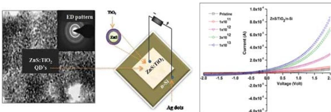
Fig. 1 (a) schematic representation of electrically connected ZnS:TiO<sub>2</sub>/n-Si QD's heterojunction, (b) *In-situ* current-voltage (I-V) characteristics of ZnS:TiO<sub>2</sub>/n-Si QD's heterojunction at different SHI fluences.
