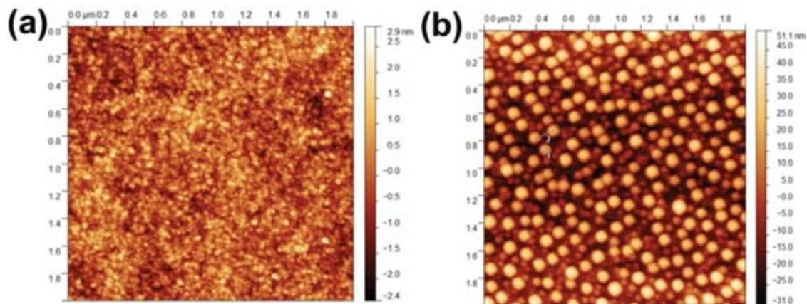
Fig. 1. The AFM image of the (a) pristine InP (100) sample and (b) irradiated sample at an energy of 50 keV
