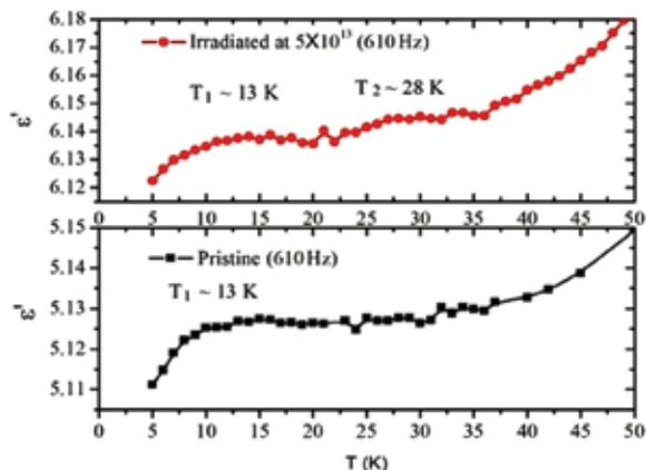
Figure 2: Dielectric constant of pristine and irradiated GdMnO<sub>3</sub> nanoparticles.
