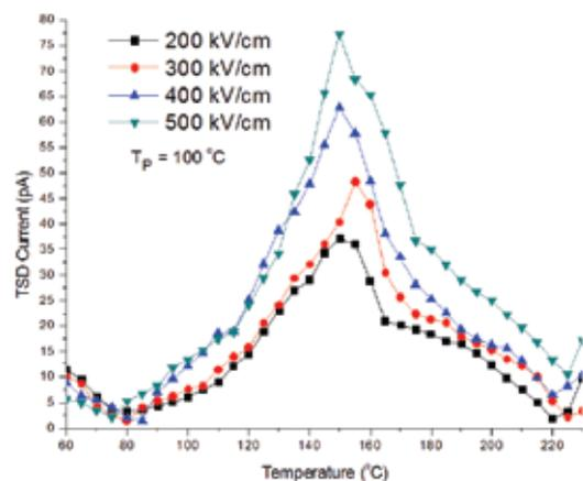
Fig. 2. TSDC spectra of irradiated PEEK
