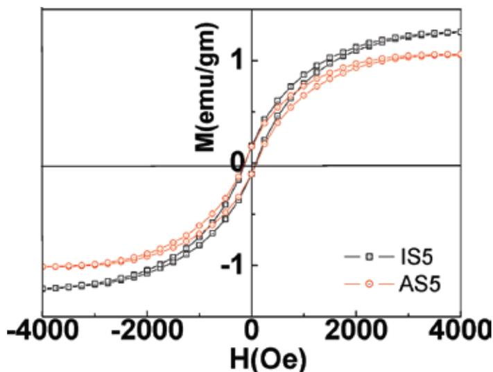
Fig. 2. M-H curves of the (a) AS, and (b) IS samples.
