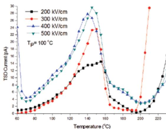
Fig. 1. TSDC spectra of pristine PEEK
