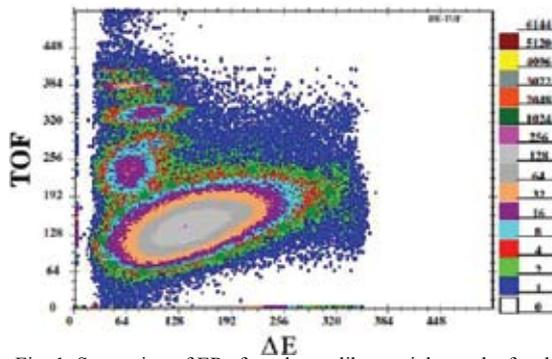
Fig. 1. Separation of ERs from beam-like particles at the focal plane of HIRA.
