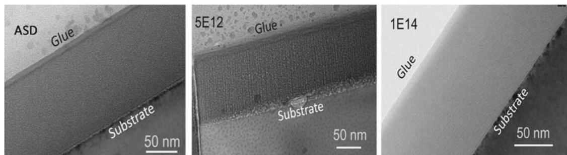
Fig. 1. X-TEM images showing the formation and dissolution of nanostructures within  $a\text{-SiN}_x\text{:H}$  matrix. Ion tracks are observed to appear at a fluence of  $5 \times 10^{12}$  ions/cm<sup>2</sup>, whereas upon exposure to a higher fluence of  $1 \times 10^{14}$  ions/cm<sup>2</sup> the tracks get dissolved due to possible overlapping.
