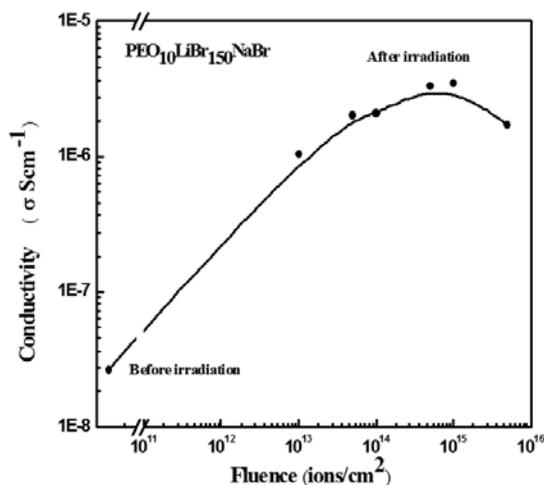
Fig. 1. Variation of conductivity of samples with irradiation fluence
