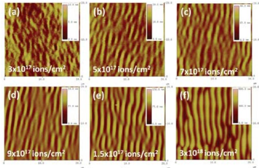
Fig. 1. AFM images of rippled patterns on Si (100) after irradiation with 200 keV Ar<sup>+</sup> at different fluences.
