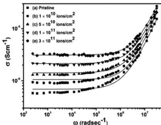
Fig. 2. ac conductivity of pristine and irradiated PANi nanofibers at fluence  $10^{10}$ ,  $5 \times 10^{10}$ ,  $10^{11}$  and  $3 \times 10^{11}$  ions/cm<sup>2</sup> at 313 K.
