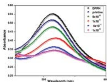
Fig. 2. Uv-Vis absorbance at 516 nm of DPPH solution in methanol after 15 min with 0.6 mg of pristine and irradiated samples with different fluences.
