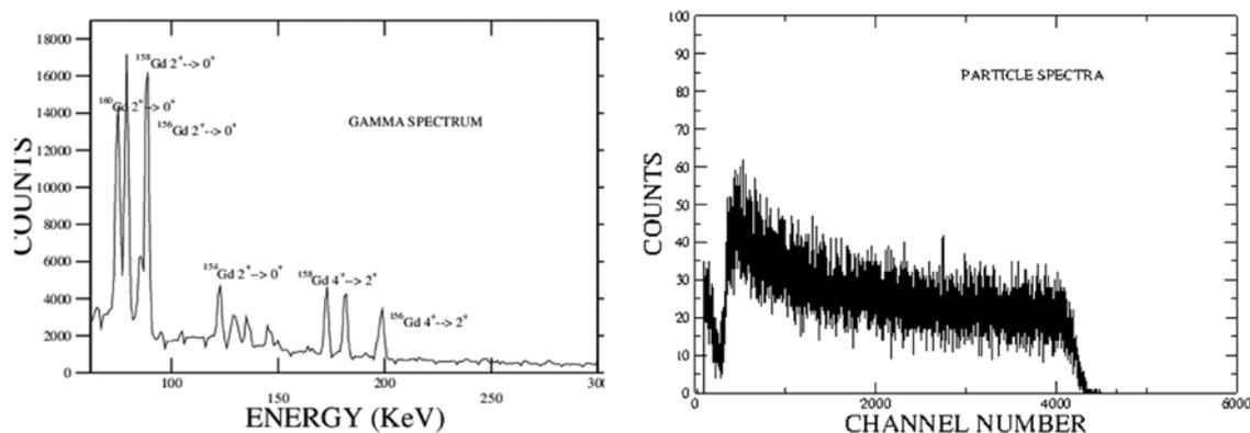
Fig. 1. Gated energy spectrum from one of the germanium detectors (left) and energy spectrum of the back-scattered  $^{28}\text{Si}$  ions detected in the particle detector (right).
