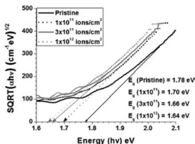
Fig. 1. Tauc's Plot of As<sub>40</sub>Se<sub>60</sub> thin films.
