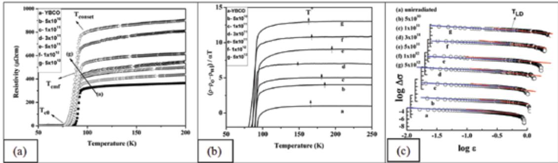
Fig. 1. (a) Illustrates dependency of resistivity on temperature for pristine and irradiated YBCO thick.
