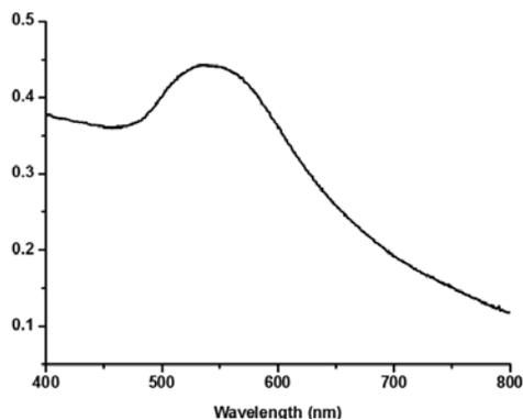
Fig. 1. UV UV-Vis absorbance spectrum of AuNP showing characteristic surface plasmon resonance peak at 540 nm.
