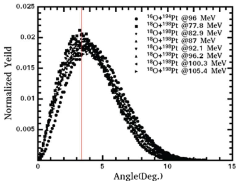
Fig. 1: Normalized ER angular distributions for  $^{16}\text{O}+^{194}\text{Pt}$  and  $^{18}\text{O}+^{198}\text{Pt}$  reactions, simulated using the Monte Carlo code TERS. The vertical line at  $3.35^\circ$  defines angular acceptance in the present set-up.
