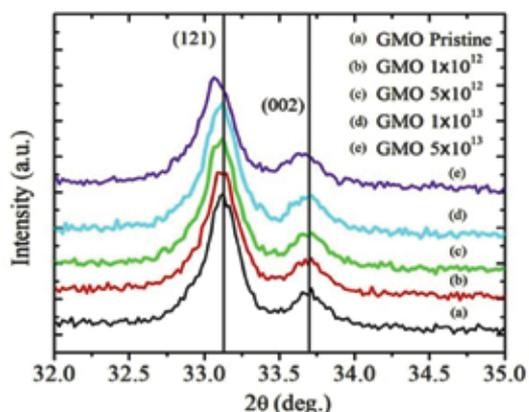
Figure 1: XRD pattern of pristine and irradiated nanoparticles of Multiferroic GdMnO<sub>3</sub>
