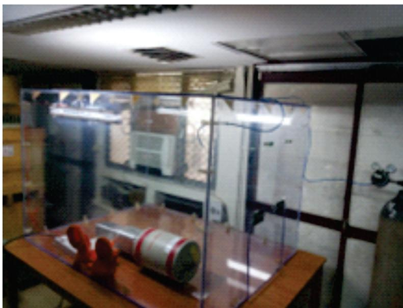
Fig. 4.2.4: Glove box for HPGe detector servicing.
