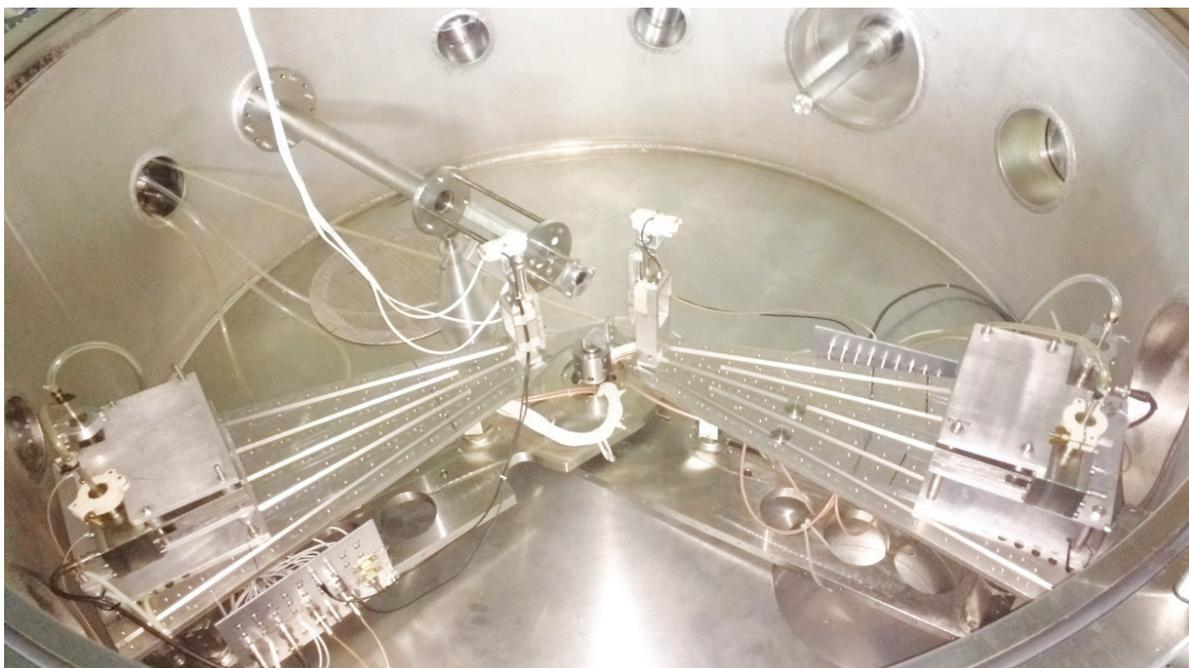
Fig.4.6.2: A setup of multi channel Doppler tuned spectroscopy
