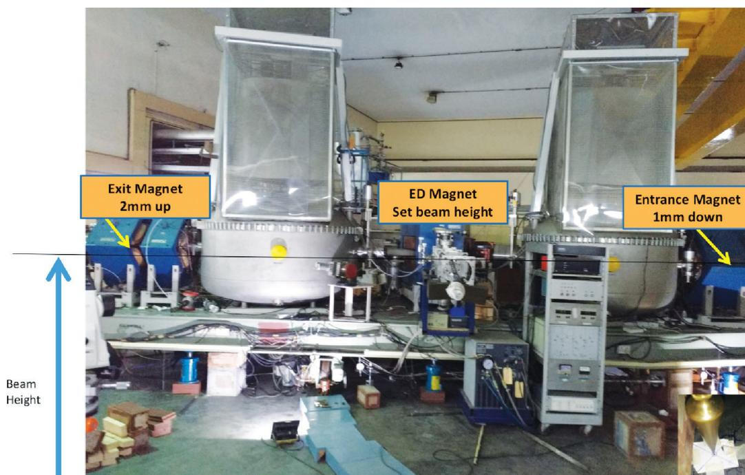
Fig. 4.3.1 Re-levelling of HIRA platform
