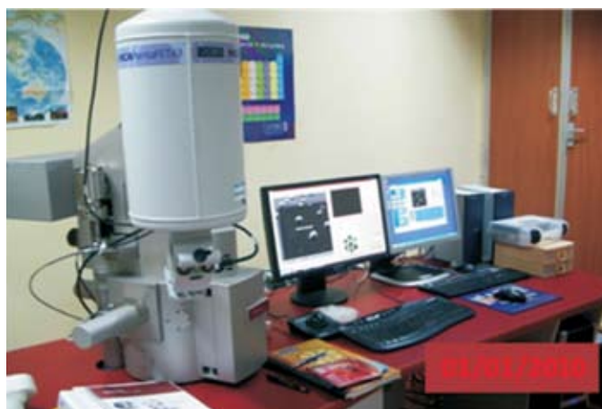
Fig.3. Tescan MIRA II LMH CS FE-SEM with Oxford INCA PentaFETx3 EDS
