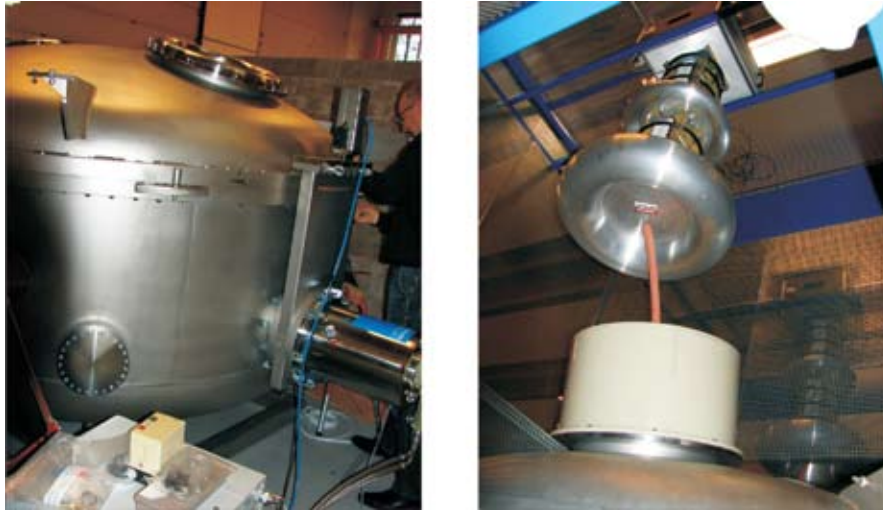
Fig. 4. (left) ED Chamber and cryo pump (right) HV supply and Faraday cage
