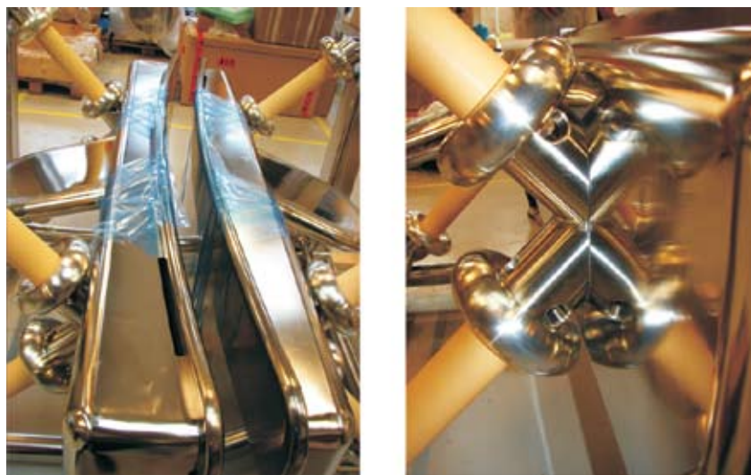
Fig. 5. (left) Electrode system (right) Backplane of electrode with support
