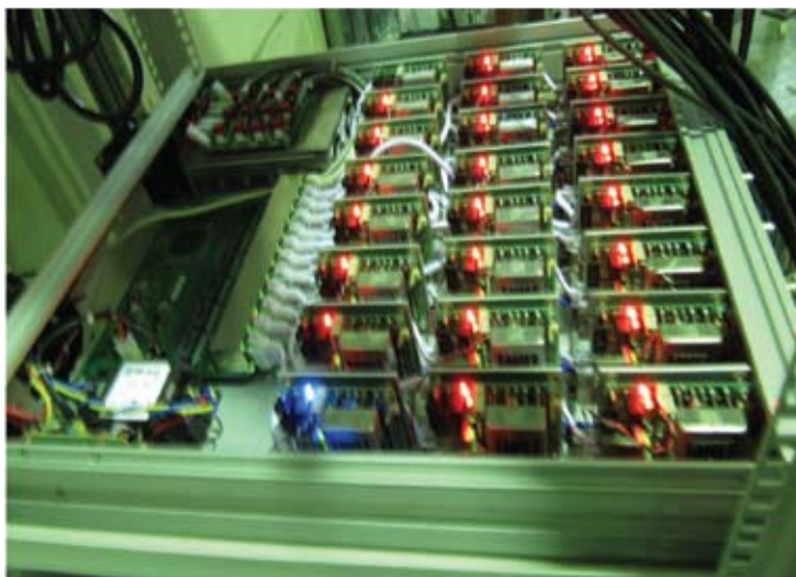
Fig. 2. High voltage power supply
