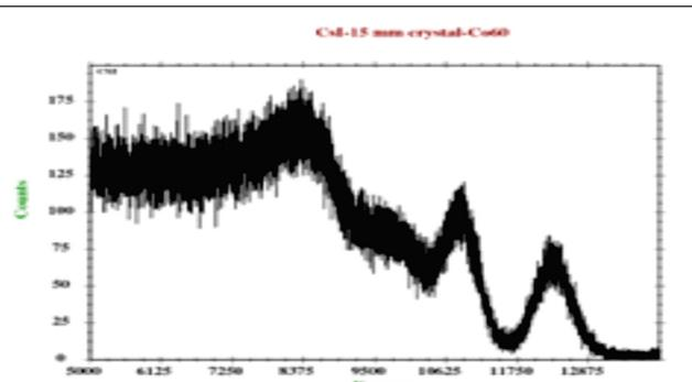
Fig.9: Co<sup>60</sup>  $\gamma$ -rays from CsI-PIN diode combination.
