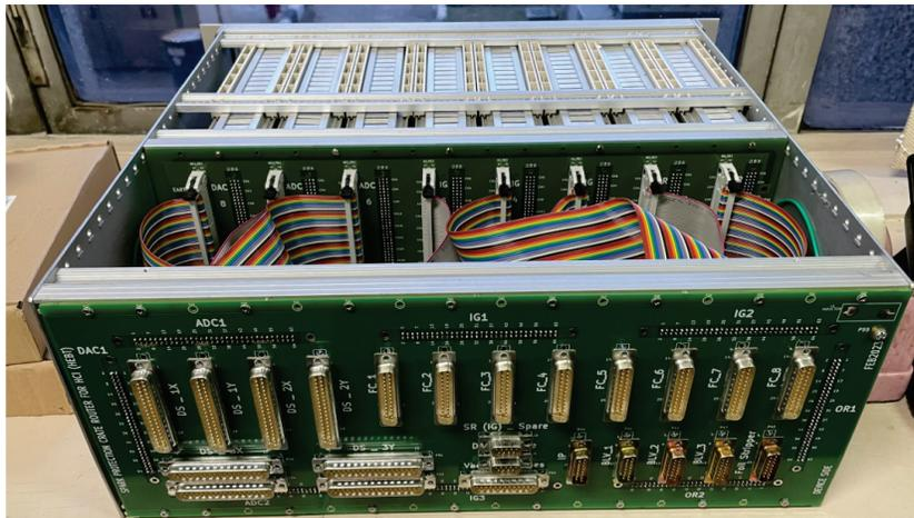
Figure 3: Spike Suppressor modular circuitry: To beam line Devices
