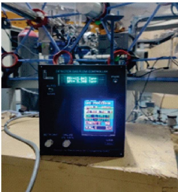
Fig. 3.1.10.5.1 A special low-overshoot Gas Pressure and flow controller under test in NAND
