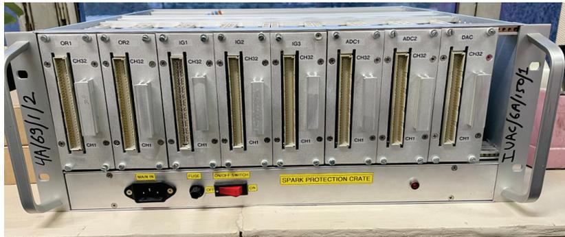
Figure 2: Spike Suppressor modular circuitry: To VME modules
