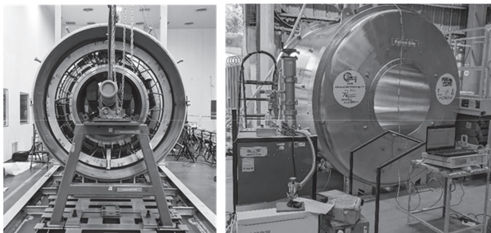
Fig. 3.1.2.2 The integration of the 1.5T superconducting MRI magnet.
