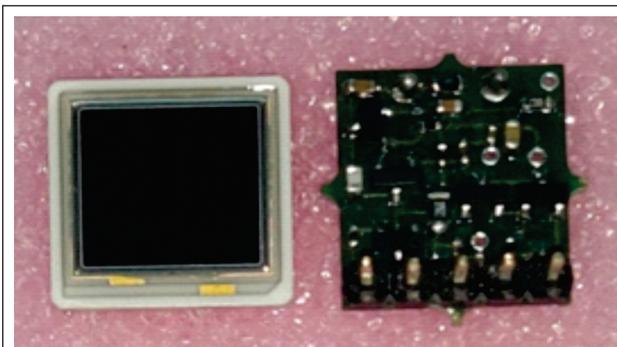
Fig.8: CSPA unit (right) with PIN diode (left)
