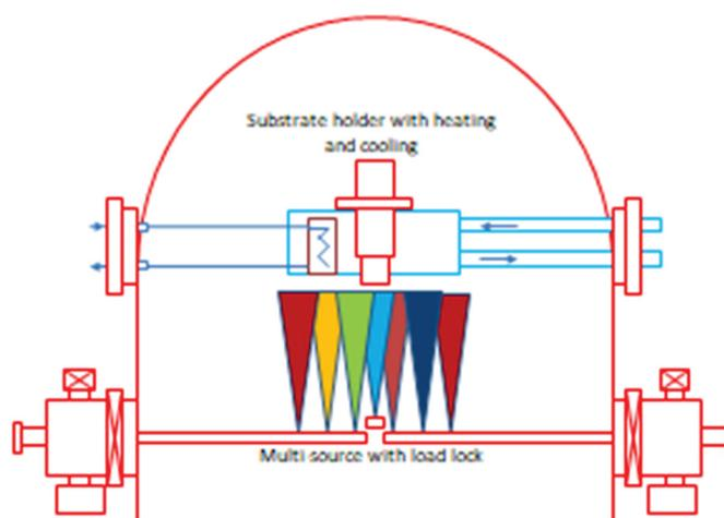
Figure 3: Photocathode deposition facility at IUAC and the schematic of source-substrate orientation
