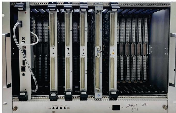
Figure 1: VME Crate system with bus controller and I/O modules
