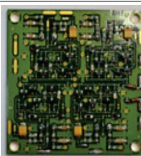
Fig.3: Four channel CSPA
