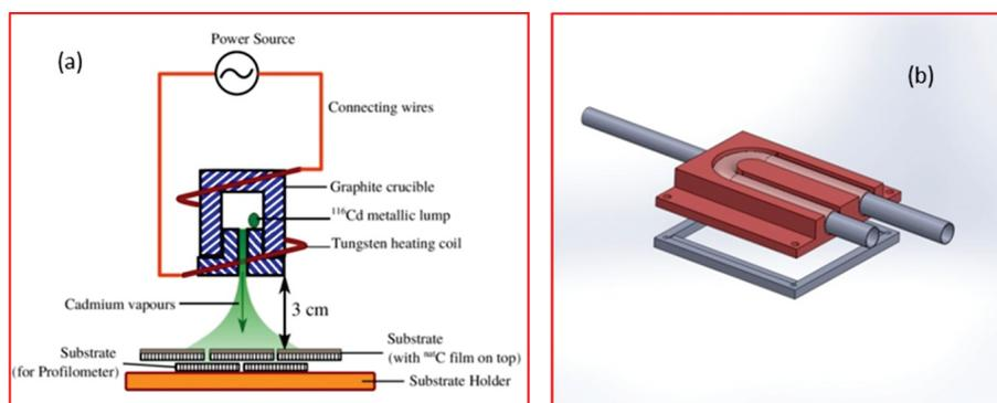
Figure 1: Schematic of (a) the Cd evaporation set-up and (b) substrate cooling set-up
