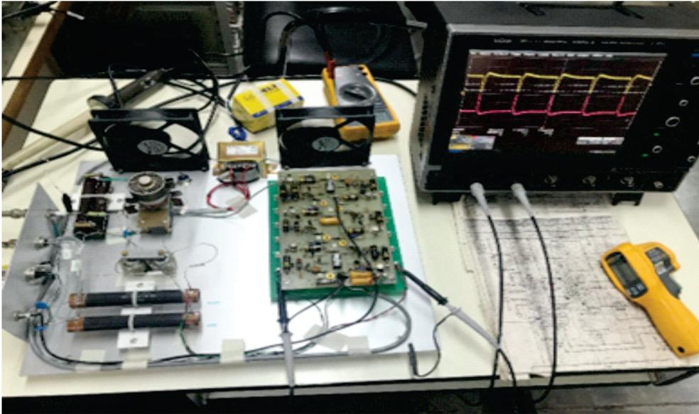
Figure 3: Test Bench for TWD Control Electronics
