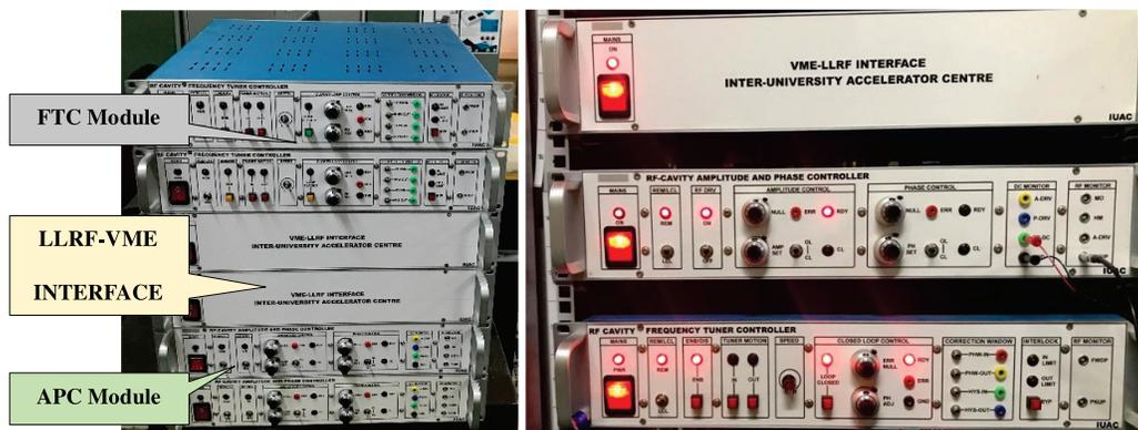
Figure 5 LLRF-VME Interface during Testing and RFQ powered remotely using the Interface
