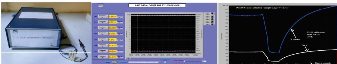
Fig 3.1.10.4.1 Pt-1000 sensor electronics, data-logger utility & calibration results
