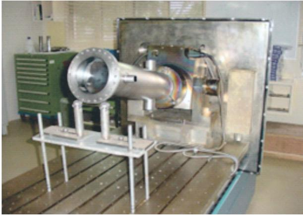
EBW set up of multi cell cavity of VECC
