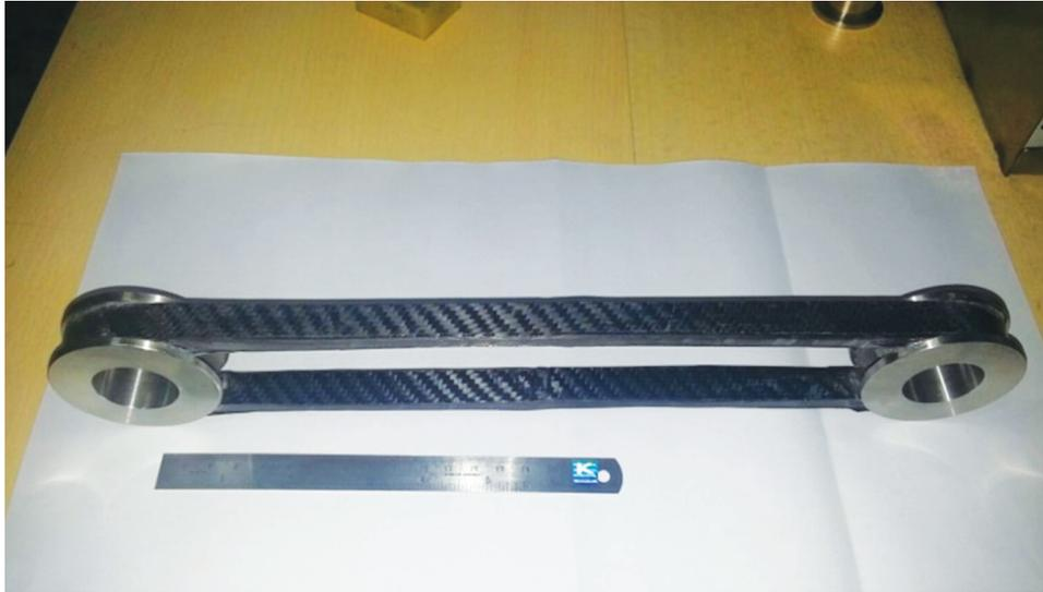
Fig. 3.1.10: Carbon fiber support with SS fixture
