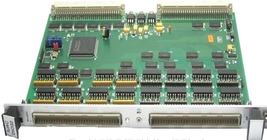
Figure 3.1.17:VME\_I64, Digital Input VME board
