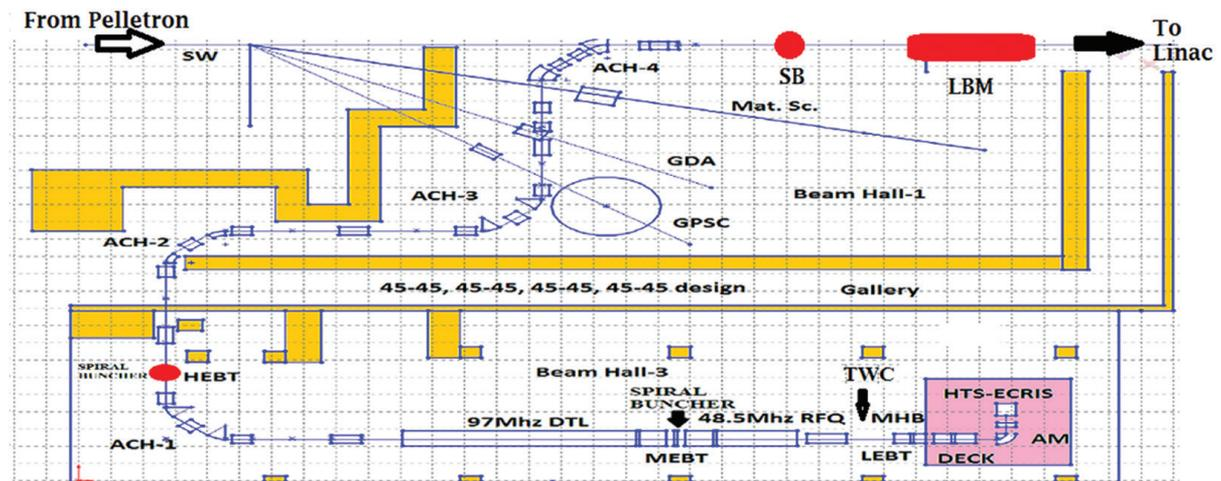
Fig. 3.1.20: IUAC HCI facility: beam hall layout
