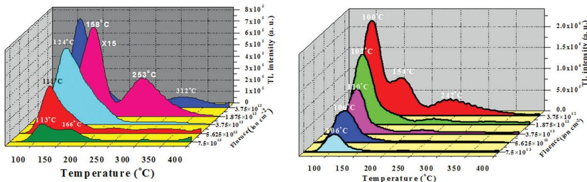
Fig. 3.1.22: TL glow curves of LiCaBO<sub>3</sub>: Ce samples irradiated by the 75 MeV C<sup>5+</sup> ion beam at different fluences
