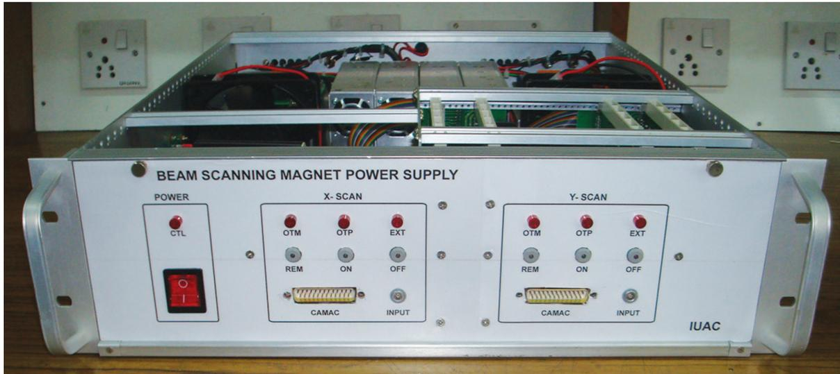
Fig. 3.1.14: Power supply unit for beam scanning magnets
