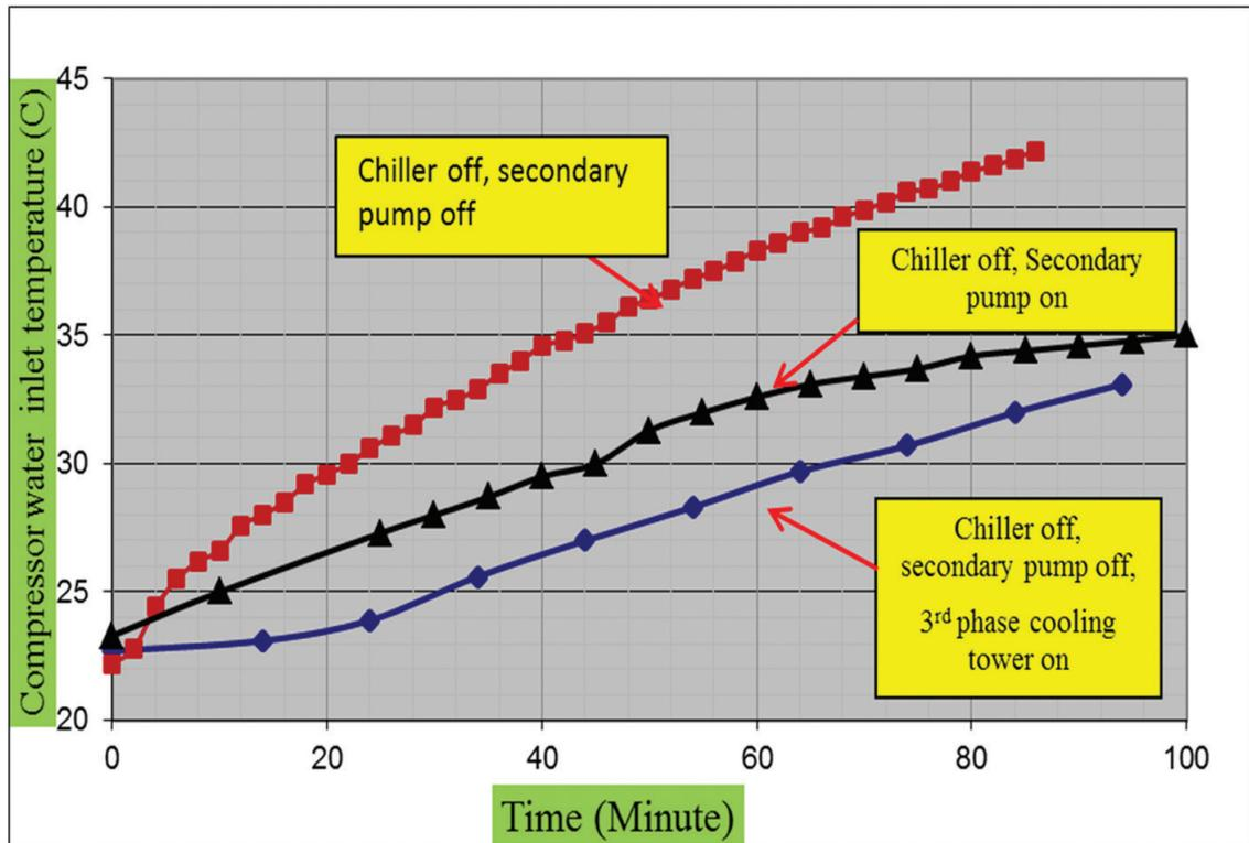
Fig. 3.1.6: Compressor water inlet temperature versus time
