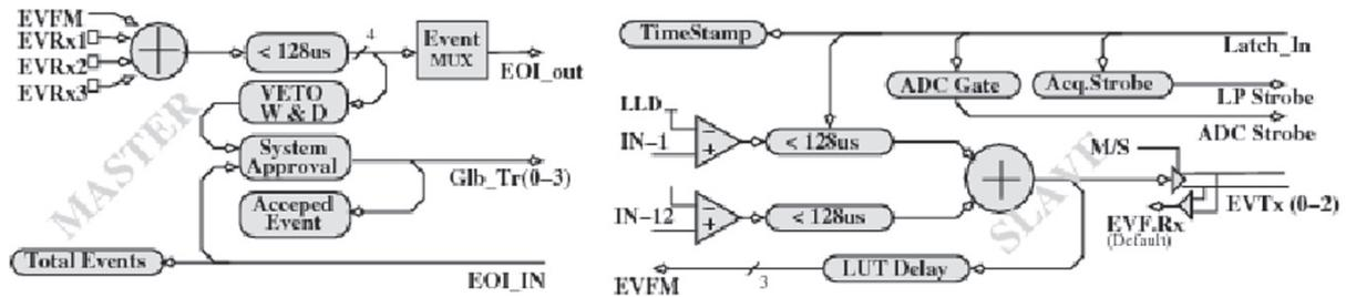
Fig. 3.1.27: Logic diagram for Event Assembly and Strobe generation
