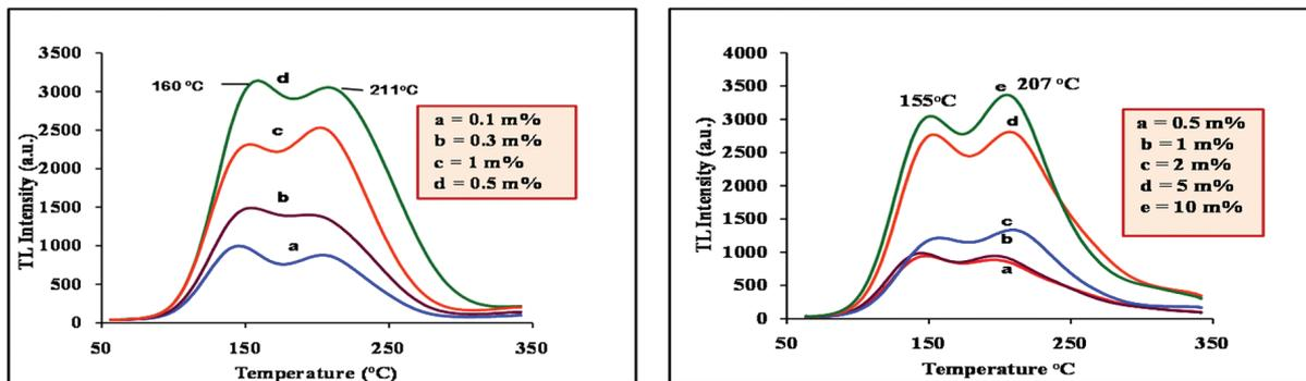
Fig. 3.1.21: TL glow curve of LiCaBO<sub>3</sub>: Dy/Ce phosphor (at gamma ray dose of 1.2 Rad).
