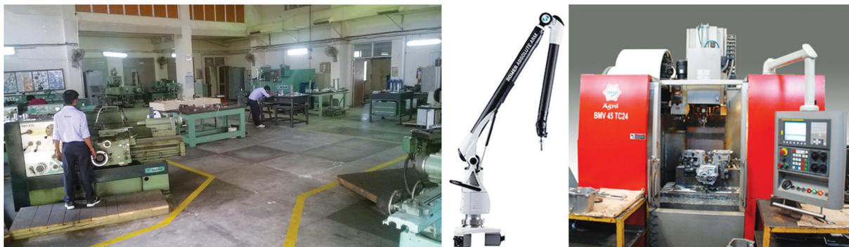
Fig. 3.2.1: (left) Machine Shop, (centre) Portable CMM and (right) CNC Vertical Machining Centre
