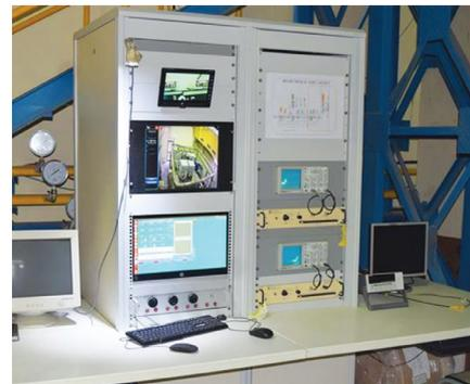
Figure 3.1.2: Control Console HCI LEBT section
