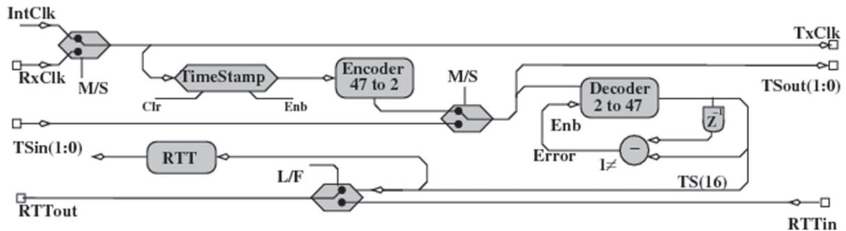
Fig. 3.1.28: Depiction of encoded daisy chained zero delay time stamp
