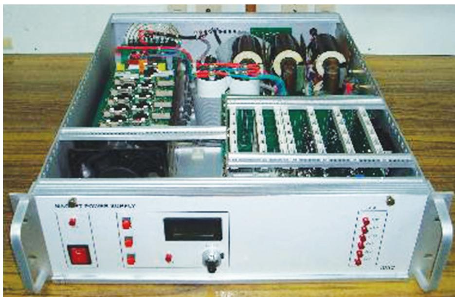
Fig. 3.1.13: Inside view of a power supply for steerer magnets
