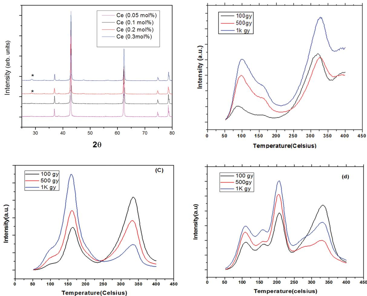
Fig. 3.1.23: (a) XRD, \* represents the CeO<sub>2</sub> phase. (b) TL of MgO:Ce (0.1 mol%) (c) TL of MgO:Li (d) TL of MgO:Ce, Li nanophosphors
