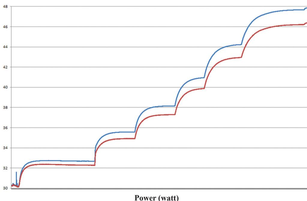
Fig. 3.1.12: Heat transfer studies with GM cryocooler in drop-in mode
