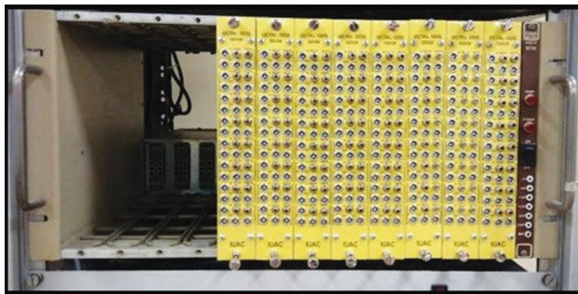
Fig. 3.1.24: Quad Logic Fan-In / Fan-Out modules for NAND Facility
