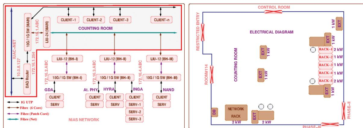
Fig. 3.1.26: (left) DAQ network and (right) Electrical diagram of counting room
