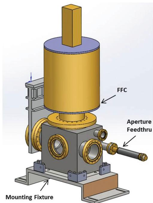
Fig. : 3.1.3: FFC Vacuum housing
