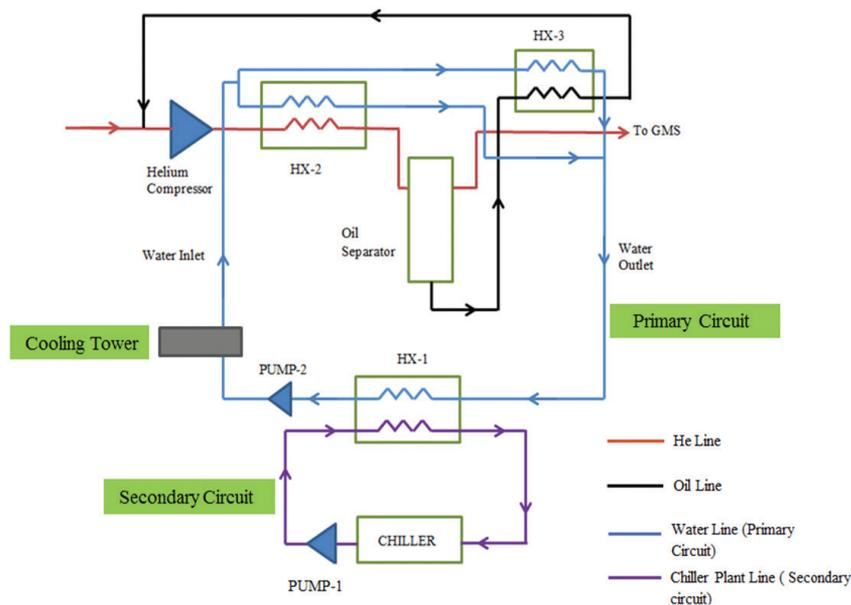
Fig. 3.1.5 : Diagram of the circuits used in the experiment to improve the compressor cooling mechanism during power failures
