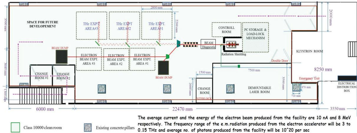
Fig. 3.1.19: IUAC FEL facility: beam hall layout
