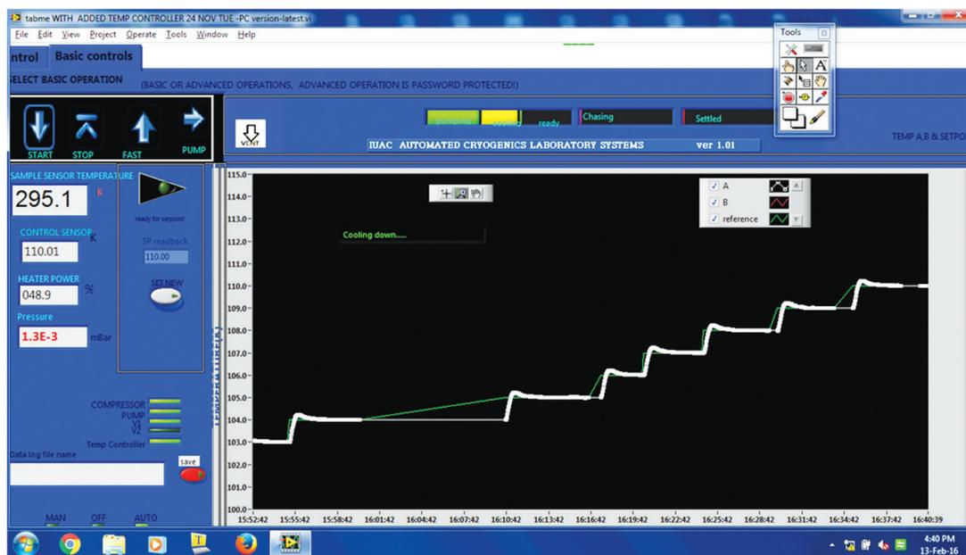
Fig. 3.1.9: Ramping control of temperature in PID mode
