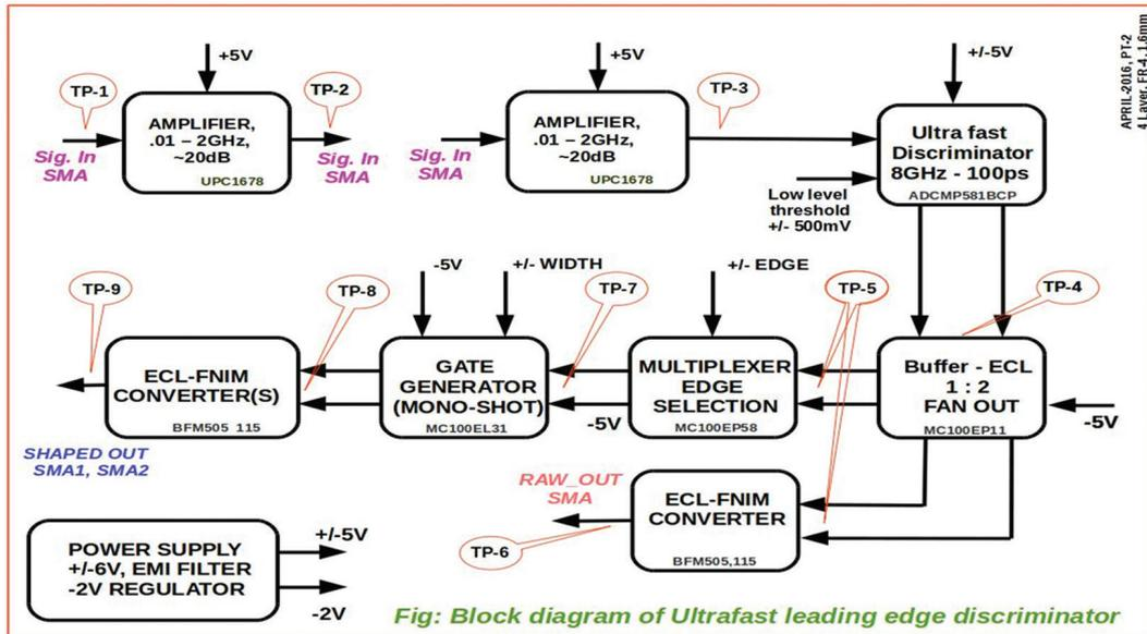
Fig. 3.1.16: Block diagram of ultrafast leading edge discriminator
