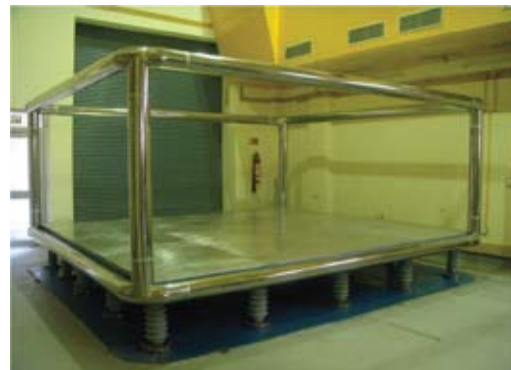
Fig 1: High Voltage Deck
