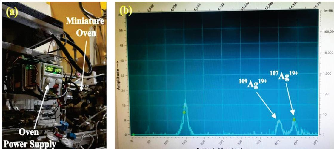
Figure 2 : (a) Micro-oven coupled at the injection side of the ECR source (b) Beam profile depicting the isotopes of Ag.
