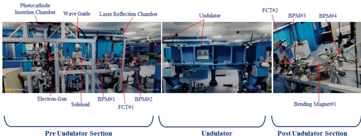
Figure 1. The complete beam line for pre and post Undulator sections along with the first Dipole magnet and the last BPM (BPM#4).
