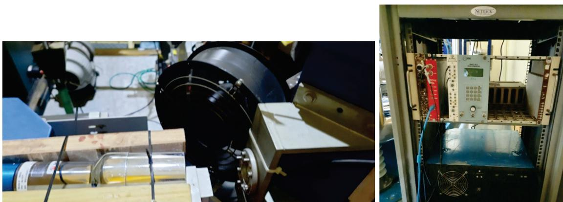
Figure 4. (Left) View of the NaI detector mounted close to the 0° port of analysing magnet and (Right) data acquisition system installed close to the 200 kV high voltage platform.
