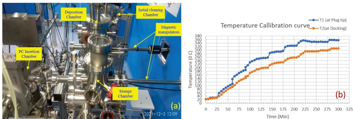
Figure 4. (a) Photograph of the photocathode deposition system installed at IUAC
