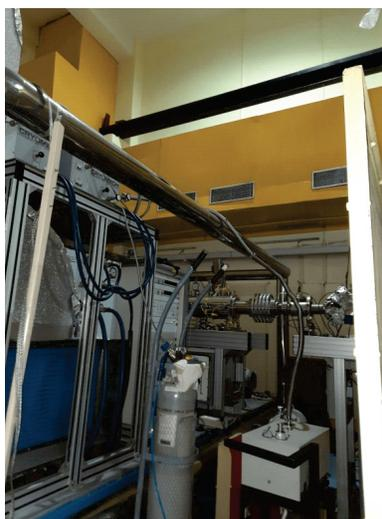
Figure 1: View of the vacuum manifold connected to extraction side cryocooler.
