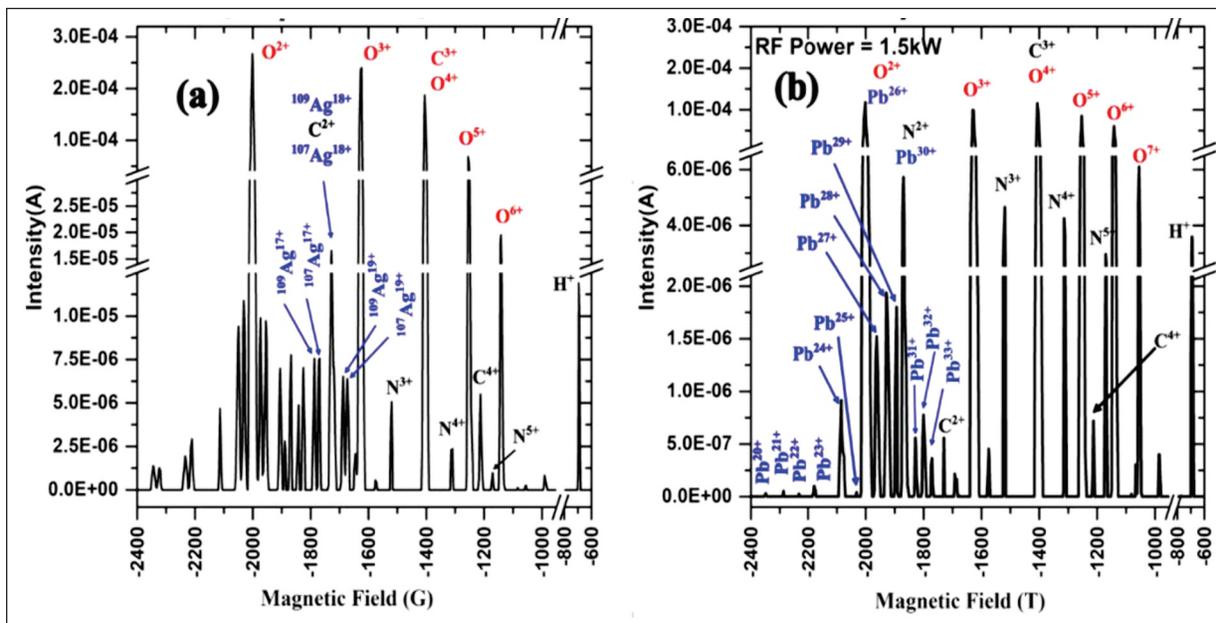
Figure 3: Charge state distribution spectra of (a) Ag and (b) Pb using  $\text{O}_2$  as mixing gas.
