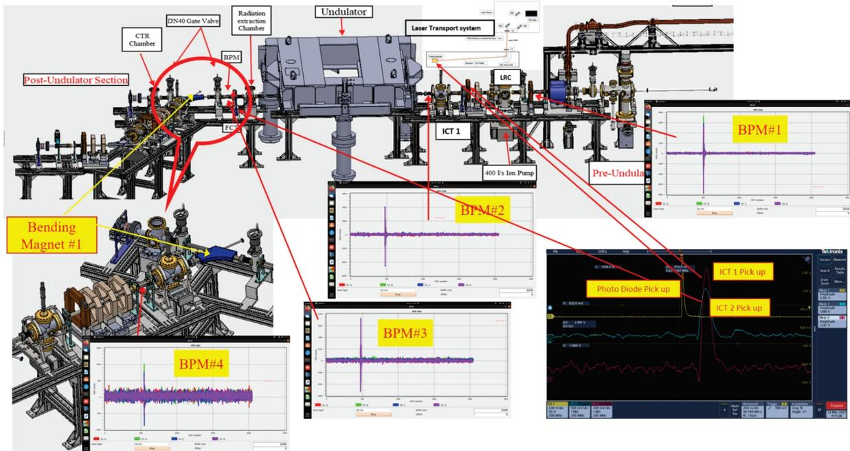
Figure 3. The complete beam line for pre and post Undulator section along with modifications for laser viewer.
