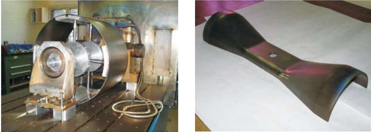
**Fig. 4. (a) Left, an Outer Shell setup for electron beam welding, and (b) Right, a Half Spoke formed in niobium.**
