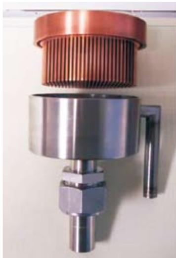
**Fig 7. The heat exchanger block of recondenser**
