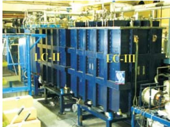
**Fig. 5. The II<sup>nd</sup> and III<sup>rd</sup> Linac cryomodules in the Linac beam line**
