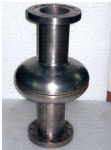
**Fig. 5. Niobium Single Cell Tesla-type Cavity. The overall height is approximately 400 mm.**
