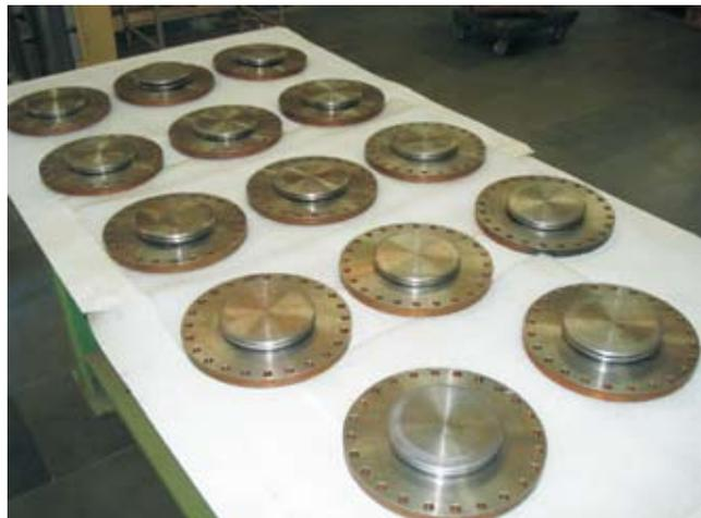
**Fig. 2. Slow Tuner Bellows assemblies**
