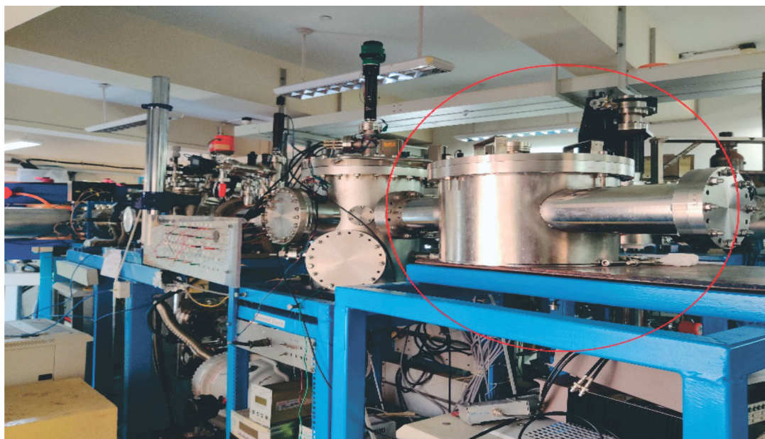
Figure 3: The post collision energy analyzer installed in 75° beam line.
