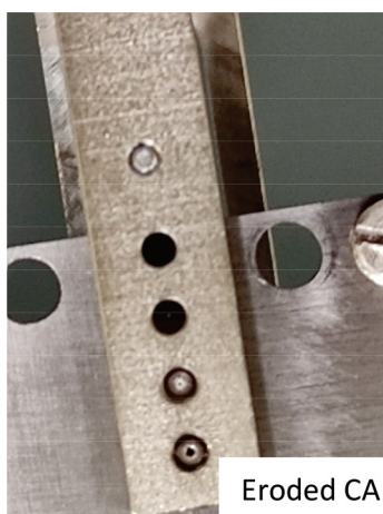
Figure 3: Eroded contrast apertures (CAs)
