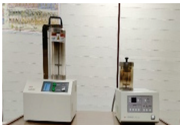
Figure 5: Carbon and Platinum Coater
