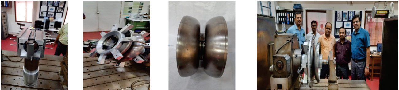
Figure 5: EBW setups showing (L to R): welding of a beam pipe, inside welding of the iris joint, stiffener ring attached to a dumbbell and outside welding of the iris joint.
