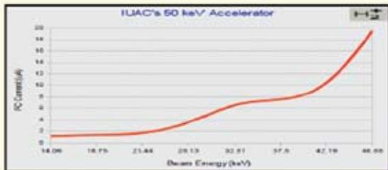
Beam Energy Vs Current at fixed Prs.
