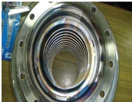
Fig. 4. Inner View of an accelerating unit. Beam marks on guard rings are clearly visible.
