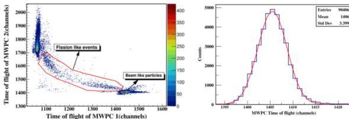
Fig. 4.1.2: Time of flight correlation of events detected in two MWPCs (left) and typical time spread of the elastic peak (right).
