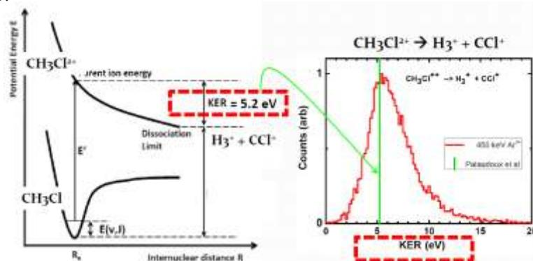
Fig. 4.6.3: Schematic representation of kinetic energy released (KER) in theoretical calculations reported in the literature (left) for the dissociation of  $\text{CH}_3\text{Cl}^{2+}$  into  $\text{H}_3^+$  and  $\text{CCl}^+$  and its verification in our experiments (right).
