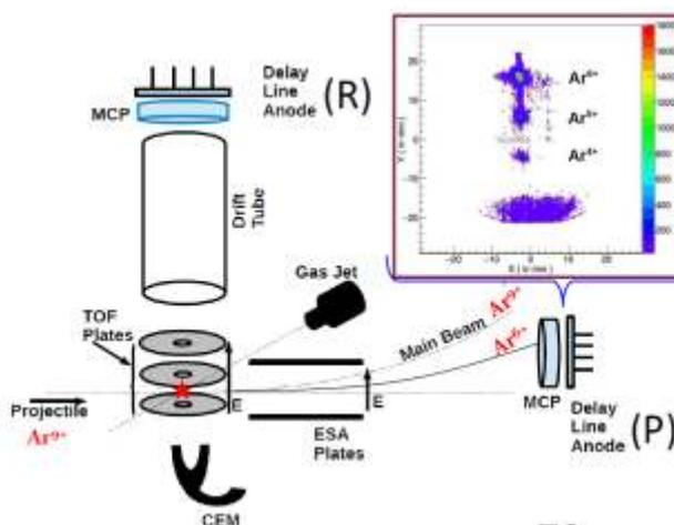
Fig. 4.6.2: Schematic of the recoil ion momentum (RIM) spectrometer with the detector for the post collision projectiles; position spectrum of the projectile ions after interaction with Ar target (inset).
