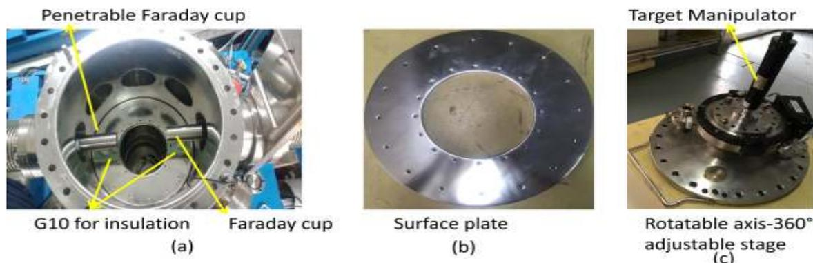
Fig. 4.6.1 Both Faraday cups inside vacuum chamber (b) Surface plate and (c) rotatable axis-360° adjustable stage.
