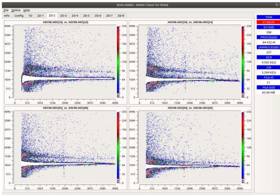
Fig. 4.1.3: MARS GUI display showing PSD versus pulse height (E) spectra for few neutron detectors during online acquisition.
