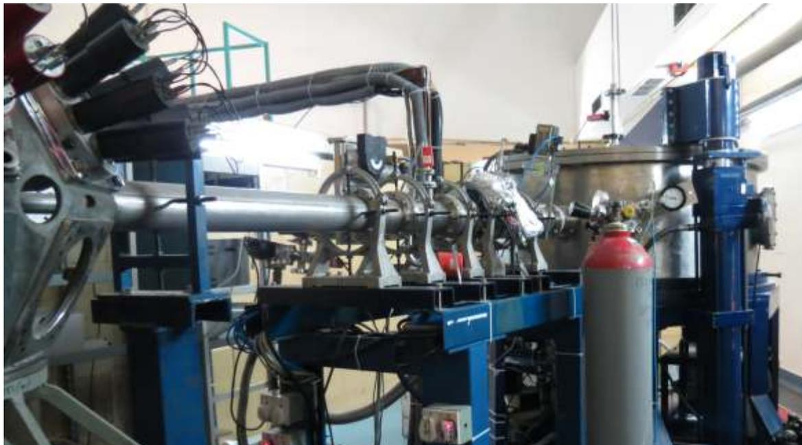
Fig. 4.1.1: The General Purpose Scattering Chamber (GPSC) installed in 30° beam line after the Gamma Detector Array (GDA) set up.
