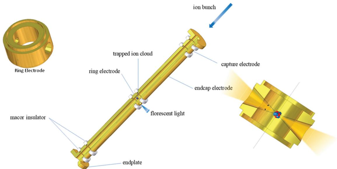
Figure 2: Section view of the ion trap electrodes assembly and ring electrode
