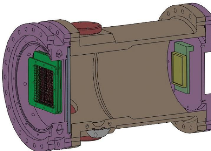
View of the planned MWPC detector and the silicon detector for detection of ERs
