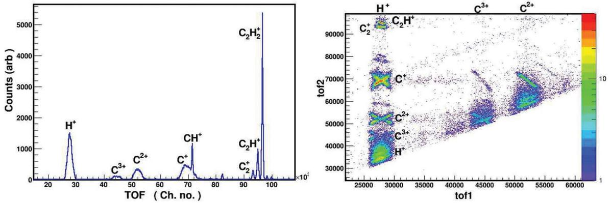
Figure 3: Time of flight spectrum (left) and double ion coincidence spectrum (right) generated in 1.8 MeV  $\text{Ar}^{9+}$  impact on  $\text{C}_2\text{H}_2$
