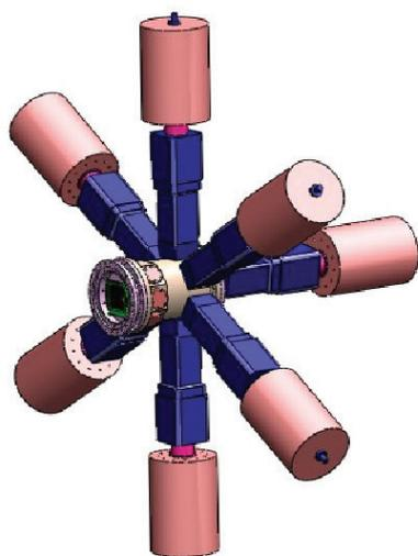
Design of new focal plane detector chamber and seven clover germanium detectors
