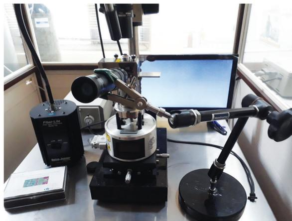
Figure 2: SPM set-up with Optical Microscope for sample viewing
