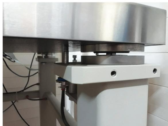
Figure 3: Vibration Isolation Table with adjusting screws
