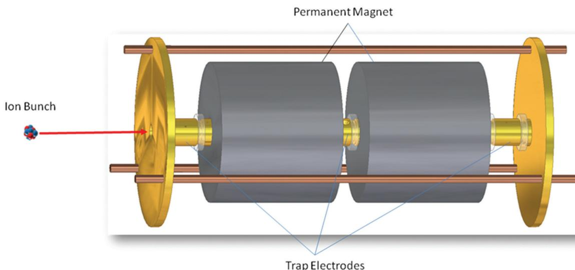
Figure 1: Schematic of the ion trap electrodes assembly with permanent magnet.
