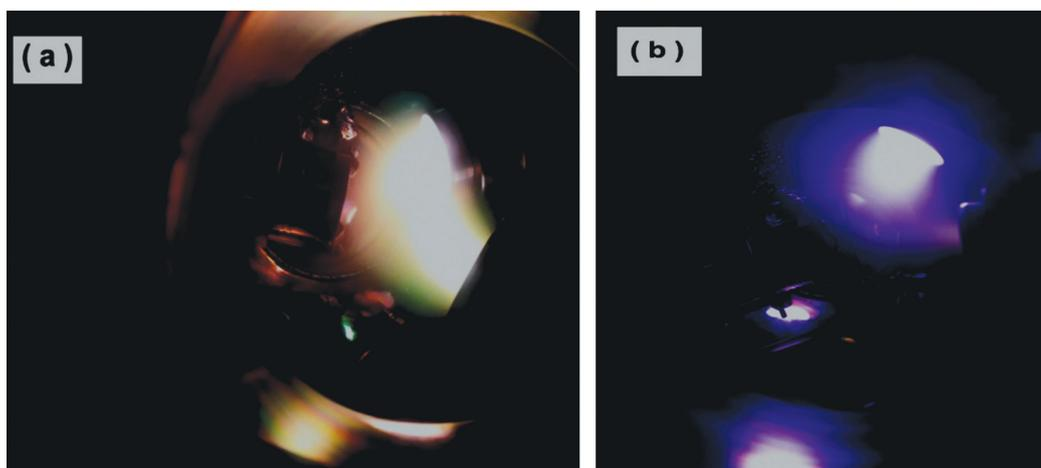
Figure: Images of plasma formed due to (a)Cu sputtering and (b) Sn , Zn sputtering.
