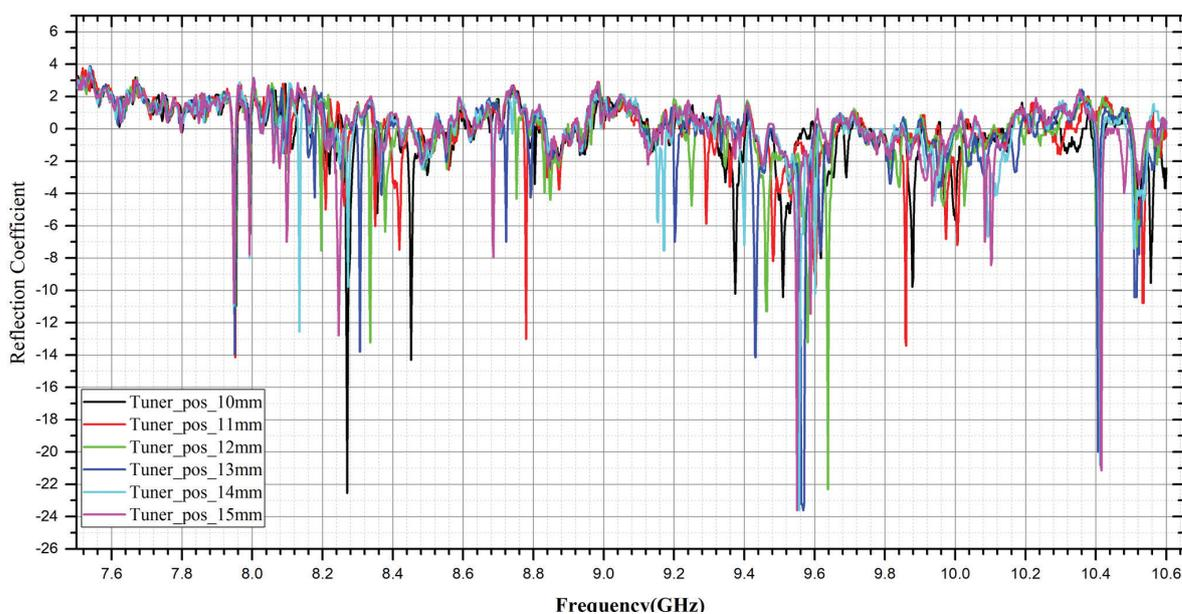
Figure 1: Reflection Coefficient at different tuner position of evacuated cavity
