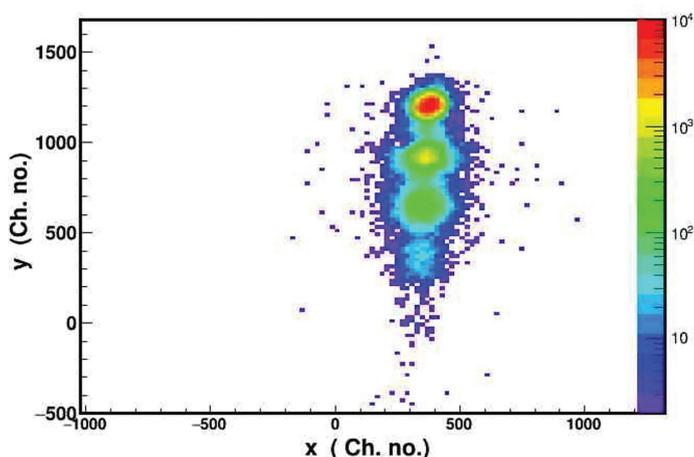
Figure 2: Position spectrum of the post collision ions in 450 keV  $\text{Ar}^{9+}$  interactions with Ar
