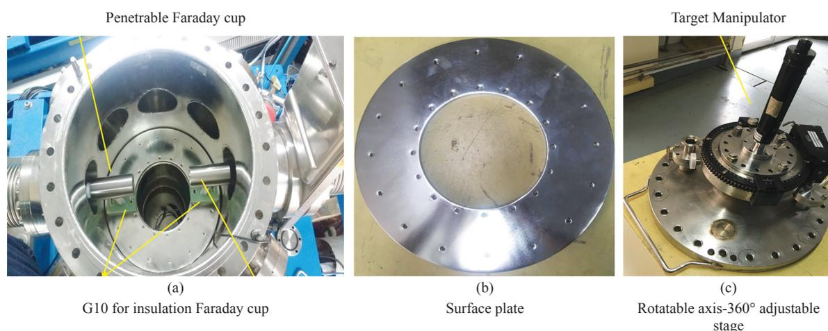
Fig 1: (a) Both the Faraday cups inside vacuum chamber are mounted on the surface plate, (b) surface plate and (c) target manipulator on a rotatable axis-360° adjustable stage.
