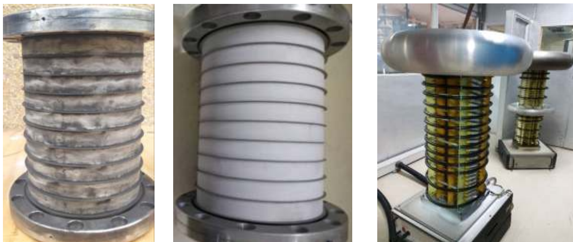
Fig 1: From left to right, dirty GP tube, regenerated tube and cleaned Cockcroft Walton Voltage multiplier stage.
