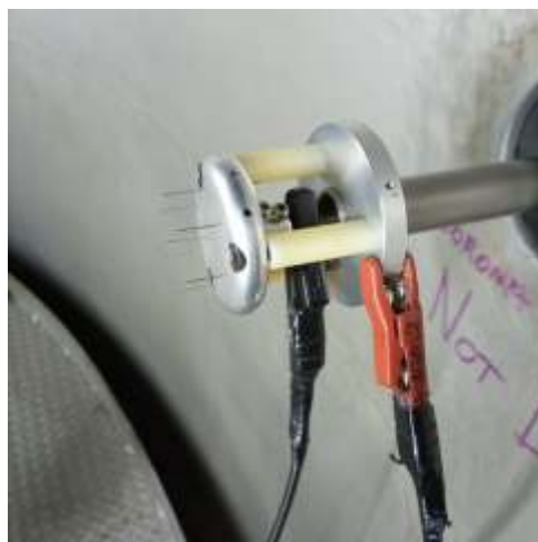
Fig 6: Corona probe insulation measurement setup.
