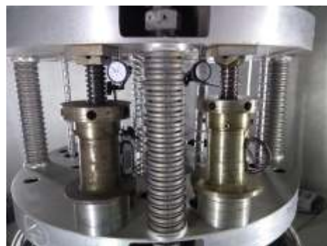
Fig 4: Column support post replacement setup.
