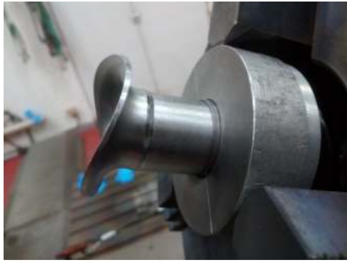
Fig 5: Electron beam welding of the niobium drift tube beam port with its saddle.
