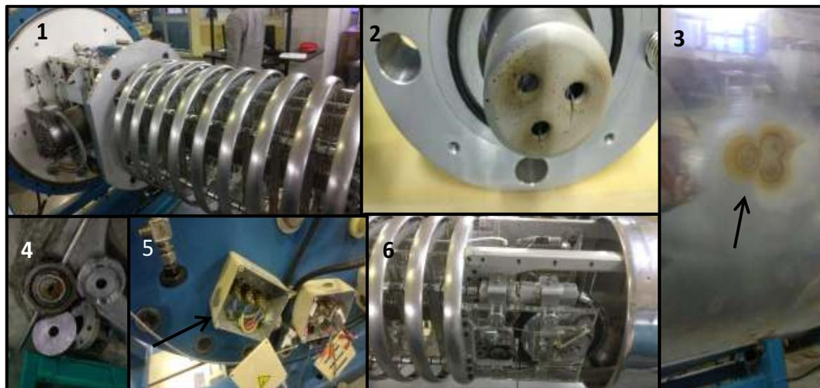
Figures: (1) Inside view of the HE section of 1.7MV (5SDH-2) Pelletron accelerator. (2) Corona probe needles and dust deposition around mushroom like head. (3) Spark marks on the terminal near to probe needles. (4) Rb choked ion source components before cleaning. (5) New chain feed through. (6) Inside view of terminal of 5SDH-2 Pelletron accelerator.
