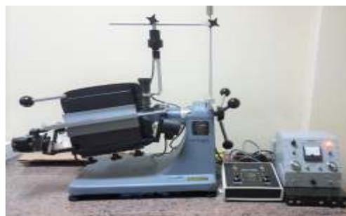
Fig. 11: Magnetic barrier separator at IUAC
