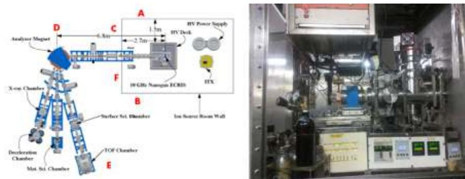
Fig. 1 (a; Left): Layout of LEIBF (top view), Fig. 1(b; Right) All-permanent-magnet 10 GHz ECRIS along with its peripheral electronics on HV platform
