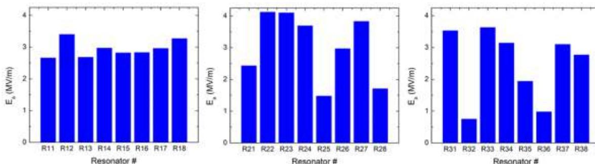
Figure 2. Accelerating gradients during linac operation
