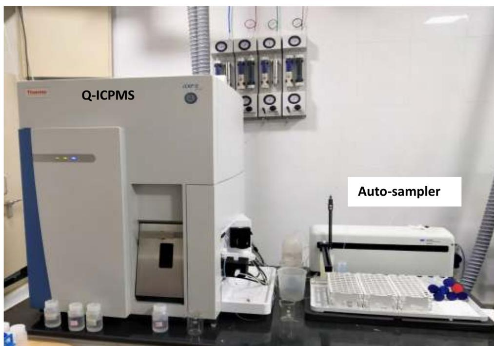
Figure 3: Q-ICPMS installed with Auto-sampler
