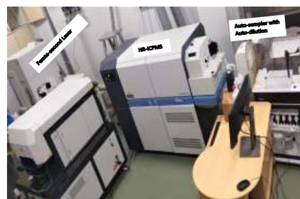
Figure 1: HR-ICPMS coupled with Fs Laser and Prefast auto-dilution system for automatic precise inline dilution (x 400)
