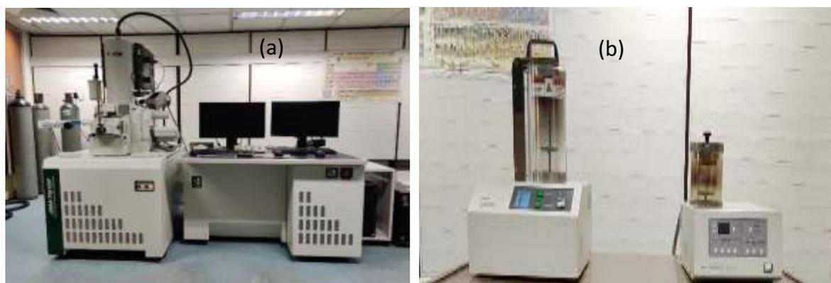
Figure 6: FESEM image (a) JEOL JSM-7610F, (b) Carbon-rod evaporator and Platinum sputter target
