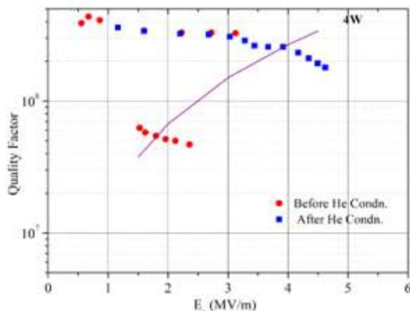
Figure 3. Q-Curves of R27 before and after Helium High Power Conditioning.
