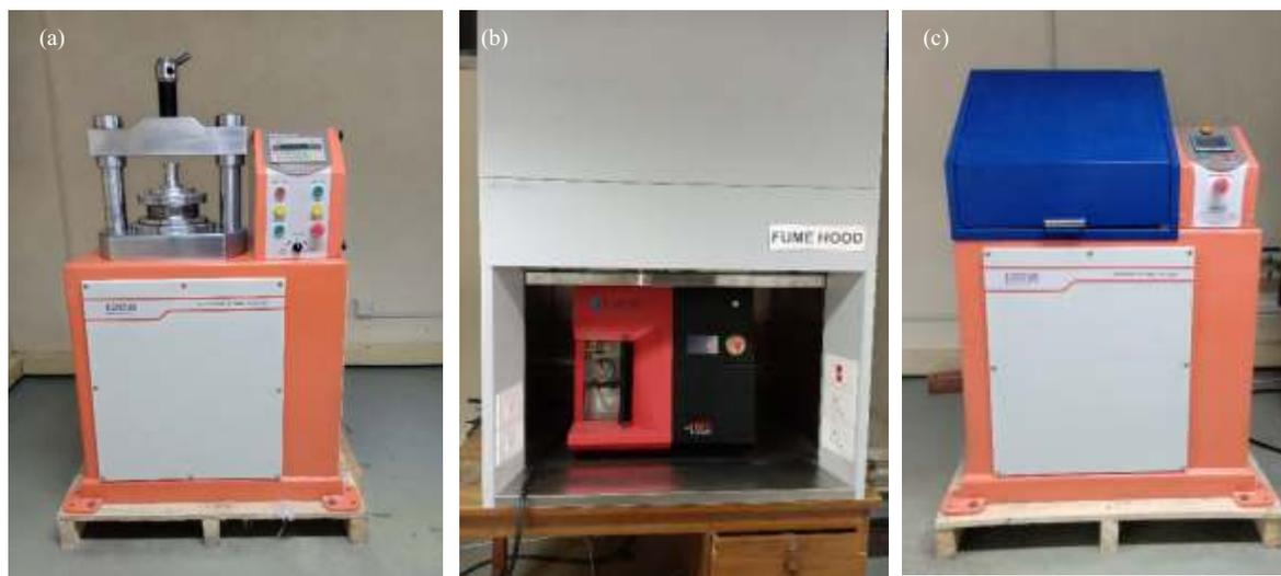
Fig: 10: (a) Pellet Press Machine (b) Fused bead Machine (c) Vibratory cup mill
