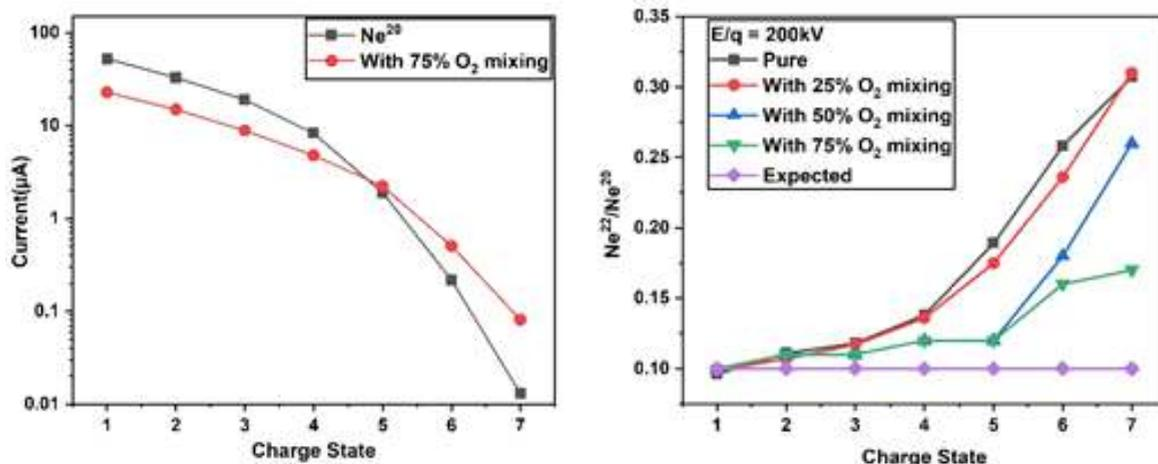
Fig. 2 (a; Left): Gas mixing effect in Ne plasma, Fig. 2(b; Right) Signature of anomalous effect in Ne plasma
