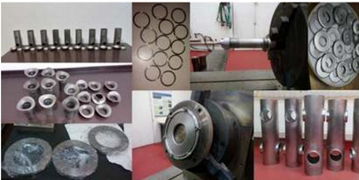
Figure 1: Clockwise from top-left: (i) elements of the niobium drift tube assemblies, (ii) weld rings for the slow tuner bellows, (iii) EBW set up for welding the drift tube beam port assembly, (iv) leaves for the slow tuner bellows, (v) SS outer helium vessels, (vi) EBW set up for welding slow tuner bellows, (vii) open-end flanges, and (viii) drift tube beam port assemblies before welding.
