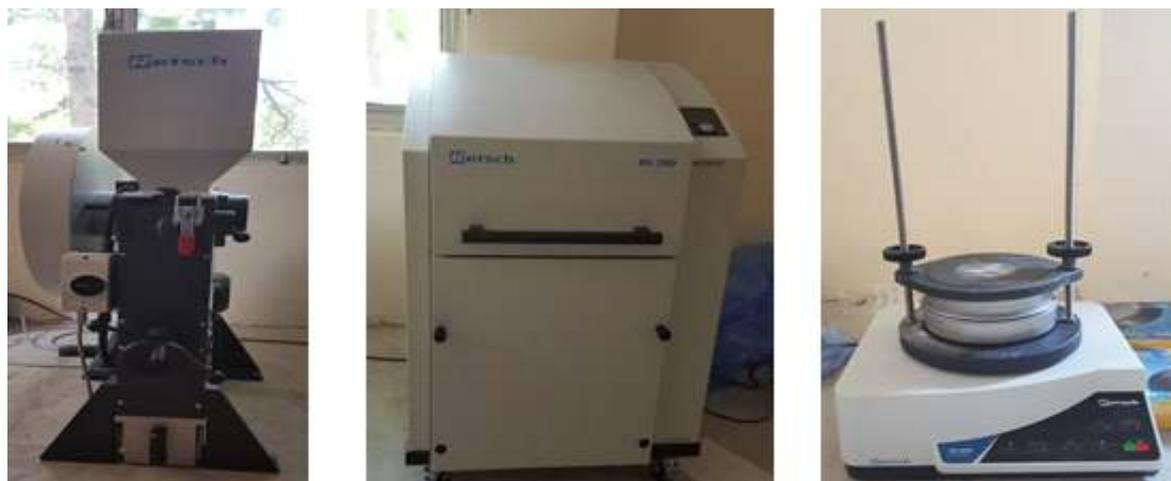
Figure 12: Jaw crusher, vibratory disc mill and sieve shaker
