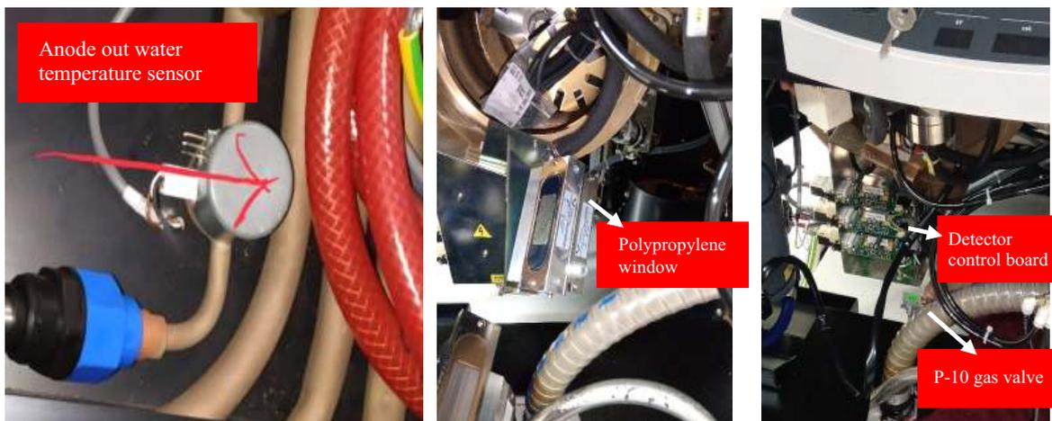
Figure 8: Replacing temperature sensor
