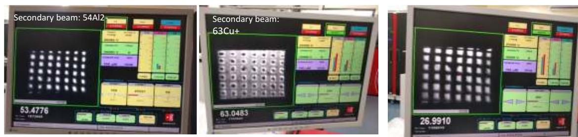
Figure 5: Direct Ion Image of Al/Cu grid using Cs+ as the primary beam and extracting  $54\text{Al}2^-$ ,  $63\text{Cu}^+$  and  $27\text{Al}^+$  secondary beam
