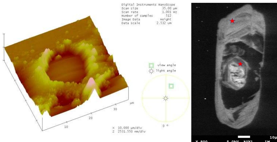
Figure 2: The AFM image of a crater created due to ablation by laser (diameter ~15 μm). A typical Zircon grain with points marked (red stars) to be ablated.
