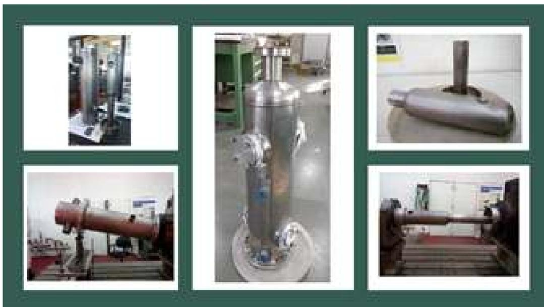
Figure 2: Centre: QWR-I11 after completion. Clockwise from top-right: (i) parts of the niobium central conductor – the loading arm with top flange (in the background) and drift tube (in the foreground), (ii) welding of the two parts of the central conductor, (iii) EBW of the niobium outer housing with the extension tube, (iv) the two major niobium sub-assemblies of the resonator before they were attached.
