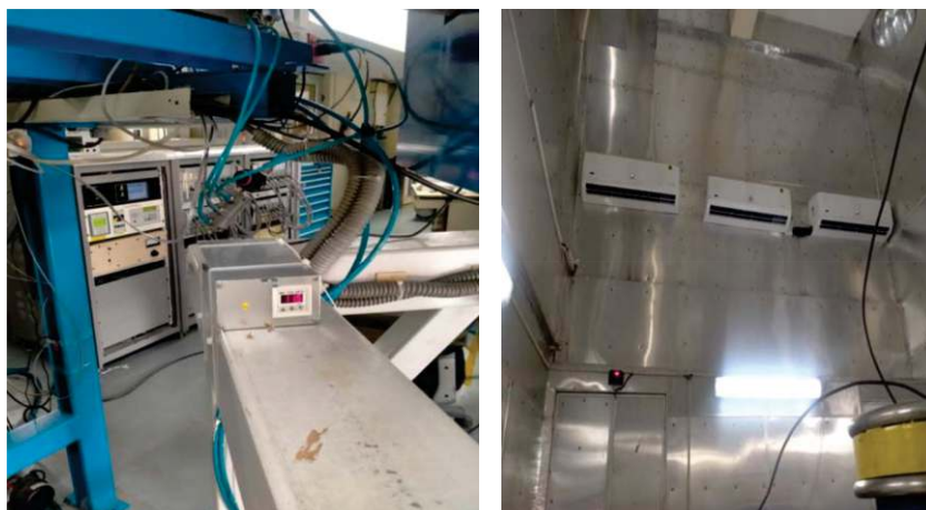
Figure 2: (a) The water flow meter installed in the beam line. (b) 3 AC units installed in the ion source room.
