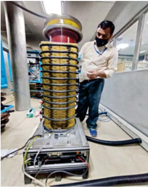
Figure 3. (a) Cleaning of Cockcroft Walton High Voltage multiplier, (b) Re-installed injector beam line.
