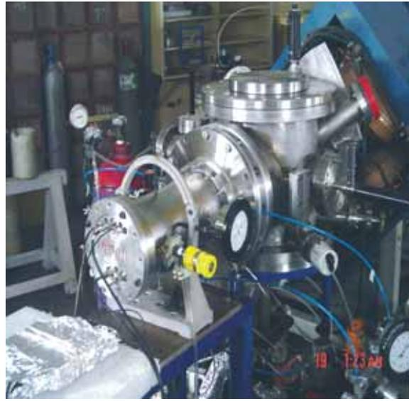
**Fig.7. IC & MWPC at HIRA focal plane**
