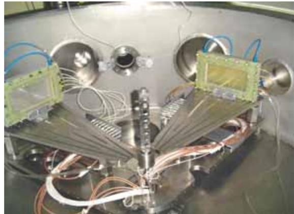
**Fig.9B. MWPCs mounted in GPSC**
