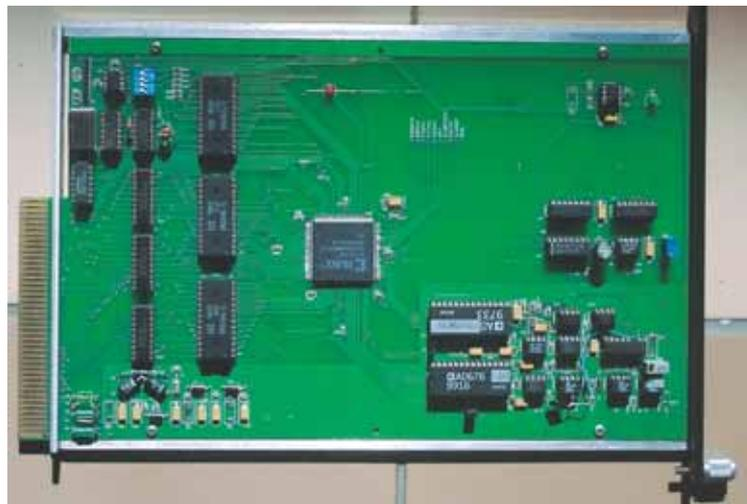
**Fig. 3. FPGA based 8K ADC with Histogram generator**
