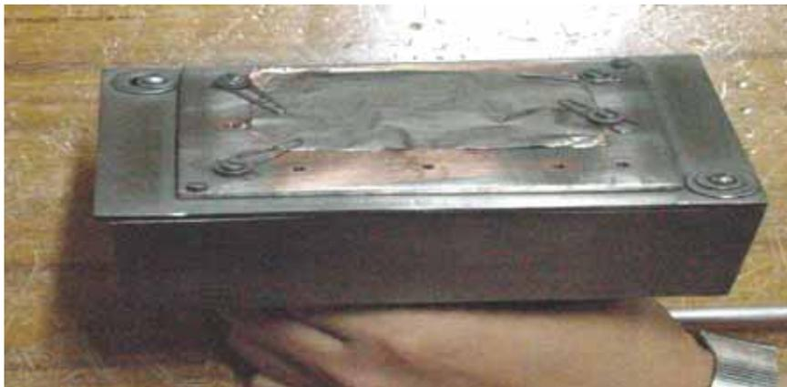
**Fig. 3. Copper mounted on substrate heater**
