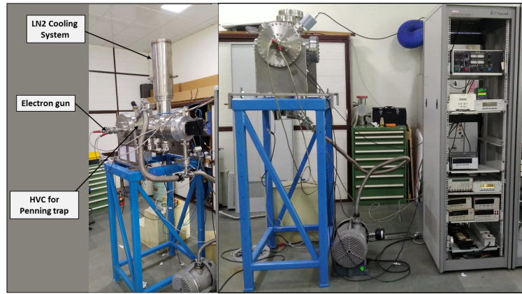
Figure 4.14: Photograph of the Delhi Penning Trap system: (left) LN 2 cooling system and electron gun integrated into the vacuum chamber; (right) complete system with diagnostic electronics and control units.
