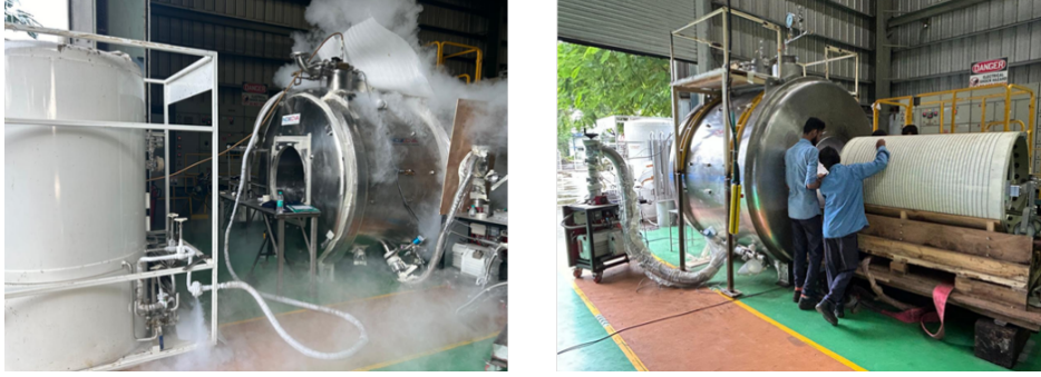
Figure 3.6: (a) MRI cryostat leak testing at 77K (b) gradient coil going into the cryostat warm bore.
