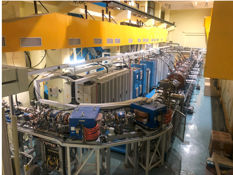
Figure 2.1: Photograph of the HCI facility at IUAC, showing major components including HTS-ECRIS, RFQ, spiral bunchers, and IH-DTL cavities.
