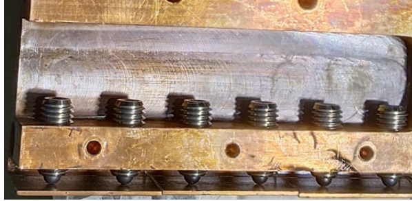
(d) Close-up of U-shaped contact pressed by plungers.
