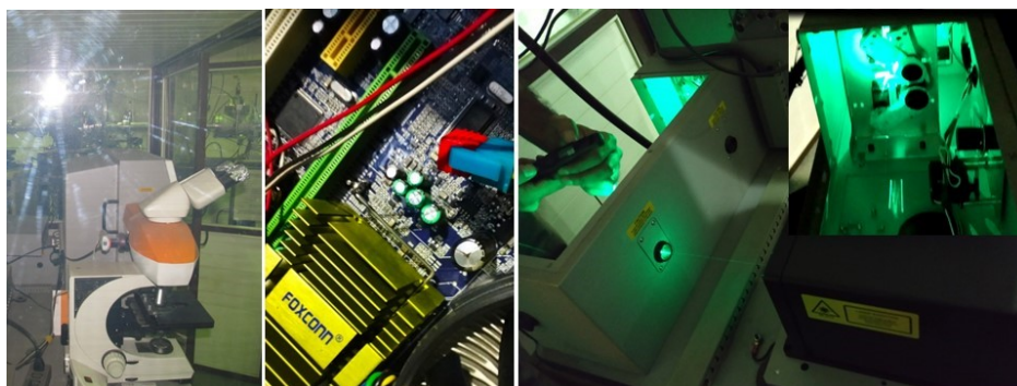
Figure 4.9: In-situ micro-Raman microscope, damaged mother board of the computer of the data acquisition and laser alignment etc. in BH-II.
