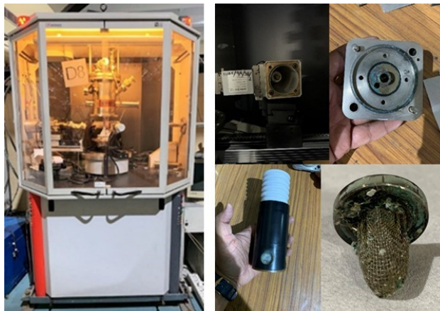
Figure 4.10: (Left) The Bruker make D8 Advanced diffractometer, a state-of-the-art in situ and low-temperature XRD machine, installed in Beam Hall-2. (Right) Illustration of the choked water filter/mesh situated within the x-ray tube of the XRD machine, hindering the cooling of the tube. Employing ultrasonic cleaning successfully cleared the obstructed mesh filter, allowing us to power the tube. The software recorded a water flow rate of 6 liters per minute during this process.
