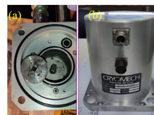
Figure 3.35: (a) Faulty cold head motor of extraction side compressor and (b) repaired motor.
