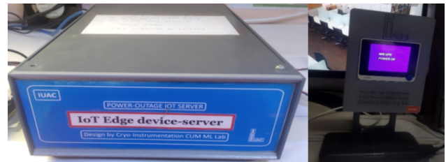
Figure 3.29: Power outage IoT edge device server and receiver unit.
