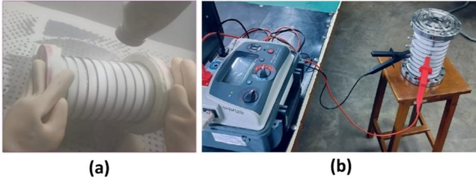
**Figure 2.7:** (a) sandblasting and (b) resistance measurement of GP tube column using a Megger.
