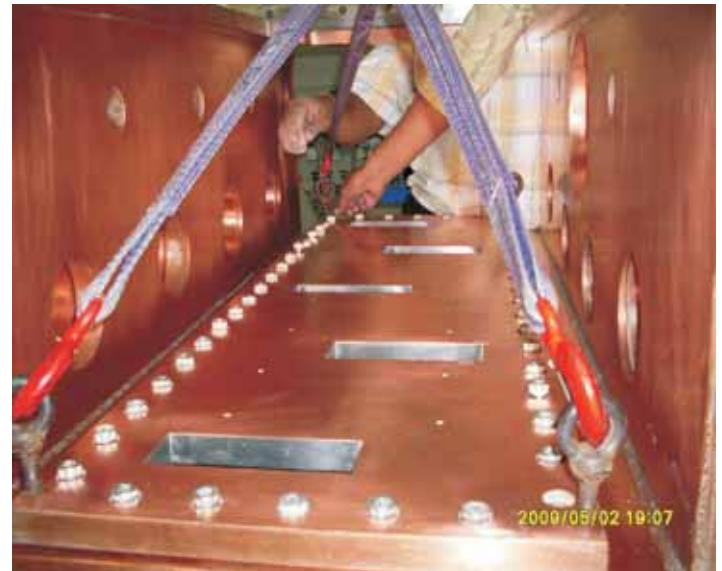
*Fig. 1. Copper plated prototype RFQ chamber*
