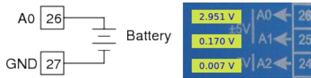
Figure 2.1: Measuring the voltage of a battery
