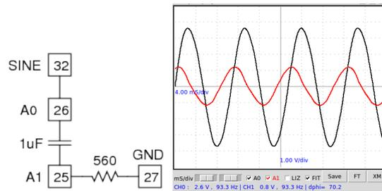
Figure 2.14: Screenshot showing the total voltage across the RC circuit and the voltage across the capacitor.  $C=1 \mu\text{F}$  and  $R = 560\Omega$ .
