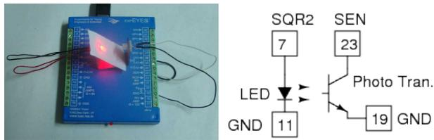
Figure 6.8: Light transmission measurement using photo transistor
