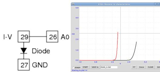
Figure 5.6: IV characteristics of Blue & Green LEDs
