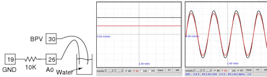
Figure 2.9: (a) Experimental setup. (b) Total DC voltage and voltage across the  $1\text{k}\Omega$  resistor. (c) Total AC voltage and voltage across  $1\text{k}\Omega$  resistor.
