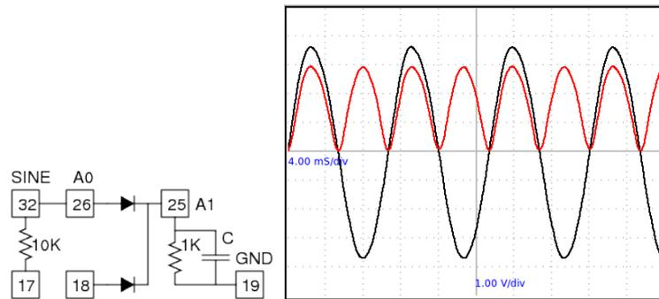
Figure 5.4: Full wave rectifier using two diodes.
