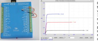
Collector and Base goes to two programmable voltage sources through 1k and 200k resistors respectively. Collector voltage is varied and plotted against collector current. This can be repeated for various base currents.
