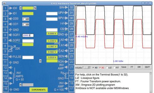
expEYES GUI demonstrating DC blocking using a capacitor.
