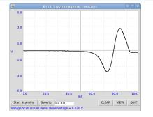
A cylindrically shaped permanent magnet is dropped in to a solenoid coil. The voltage induced across coil due to the changing magnetic field is shown above..
