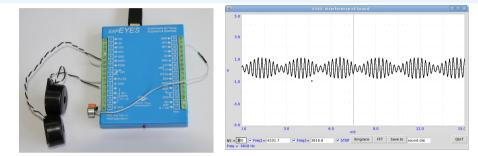
Two Piezo electric discs are made to generate sound having nearby frequencies. The resultant sound is captured by a microphone to show the beats.
