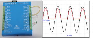
The black trace shows the direct sine wave. The red trace shows the output after passing through a PN junction diode. A load resistor of 1kOhm is connected from output to ground.
