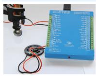
A mild steel ball is held by an electromagnet at a known height. It is released under software control and the software also senses when it hits the bottom surface. This is done by sensing the vibrations, using a loudspeaker. Acceleration due to gravity is calculated from the time of flight and the height. Time of flight is measured within an accuracy of one millisecond.
