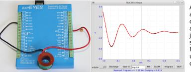
A step voltage is applied to an LC circuit. The voltage across the capacitor just after the step is shown above. Figure shows the under- damped case.
