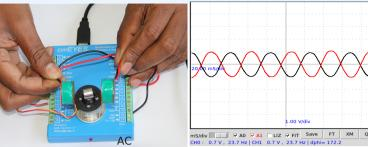
A rotating magnetic field is generated using a permanent magnet and a DC motor. The phase difference between the two voltages depends on the angle between the coils.
