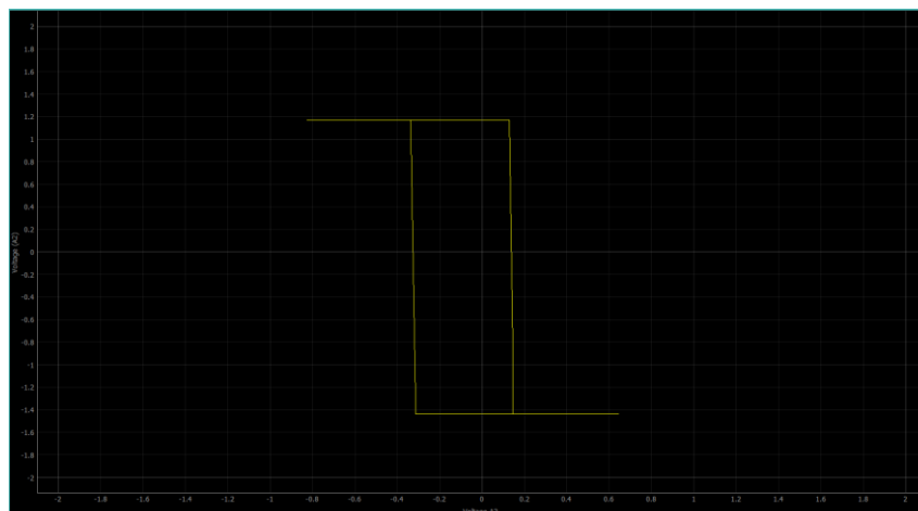
Figure 2(a): Output hysteresis loop captured on the ExpEYES oscilloscope/plotting interface
