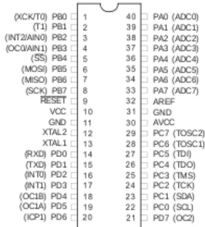
Figure 1.1: (a)Atmega16 pinout.
