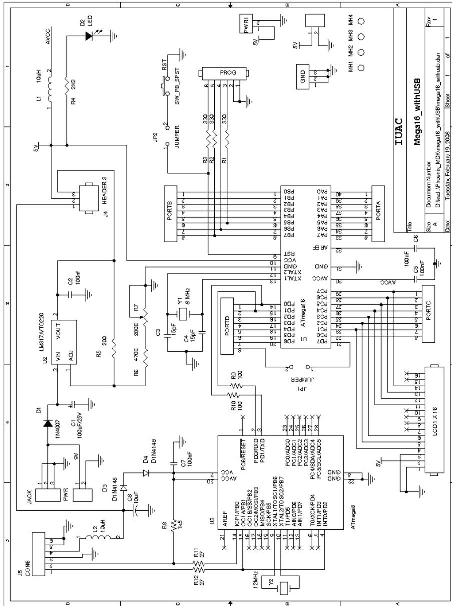
Figure 2.4: PMDK-USB schematic. The communication to the PC USB port is done through the USBtoSerial converter implemented using ATmega8.
