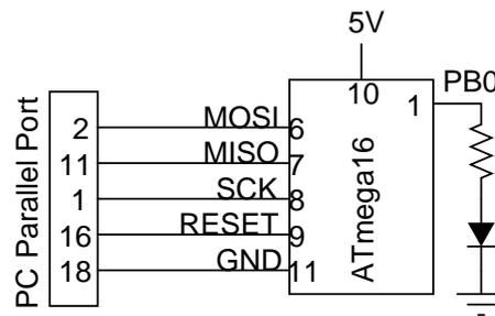
Figure 1.2: The minimum circuit required to get started.
