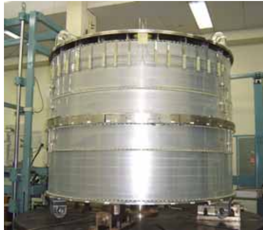
Superconducting coils wound on SS bobbin
