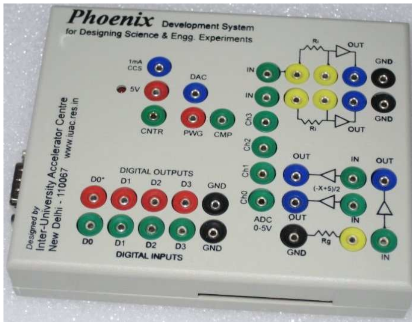
Figure 3: Photograph of Phoenix Interface. The front panel sockets having functions like Digital Input/Output, Analog Inputs (ADC), Analog Output (DAC), Waveform Generator, Frequency Counter, Op-Amp based gain blocks etc. are marked.
