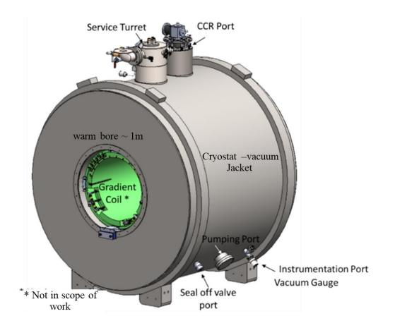
Figure 1. 3-D CAD model of the MRI cryostat.
