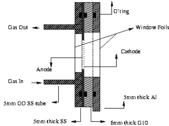
**Fig. 2 : Cross sectional view of PPAC**
