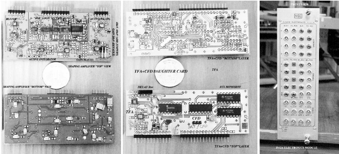
**Fig. 4 : Clover Electronics module (left) spectroscopy amplifier board (middle) TFA & CFD board (right) front panel**
