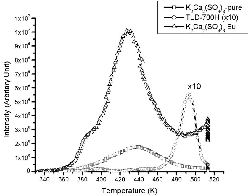
**Fig. 5 : Comparison of TL-glow curve for different samples**
