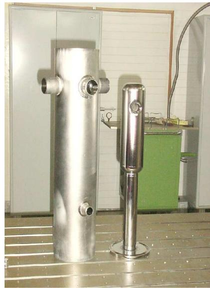
**Fig. 6 : Top Flange to Central Conductor Welding setup**
