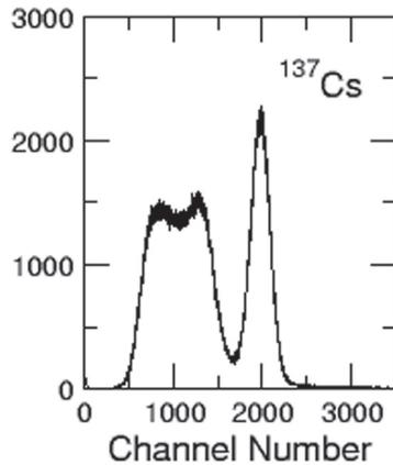
Fig. 4.2.5: Gamma Source- $^{137}\text{Cs}$ , resolution at 0.662 MeV is 12.6%.
