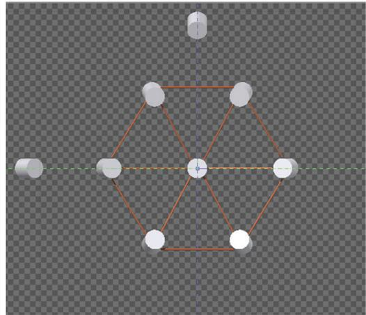
Fig. 4.1.2: Geometry used in simulation. The reference detector at the centre and the first ring of detectors is shown. The two detectors shown at far positions are part of the second ring.
