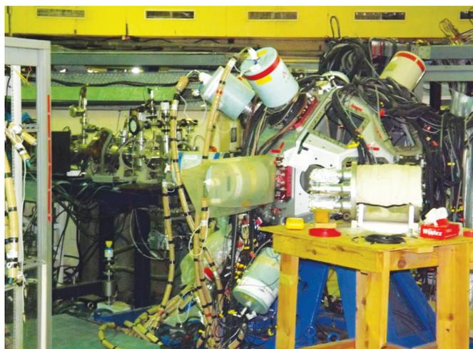
Fig. 4.2.1: INGA setup during the test run in April 2016. Fourteen Clover detectors were mounted on the back hemisphere of the INGA stand.
