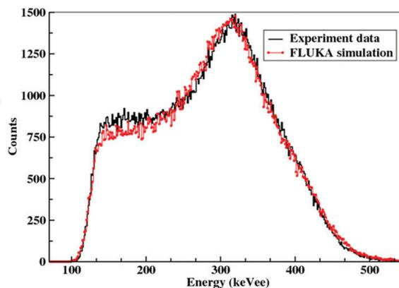
Fig. 4.1.4: Comparison of experimental light output spectrum (black line) from BC501A for 511 keV gamma rays with FLUKA simulation (red line) for 120 keVee threshold.
