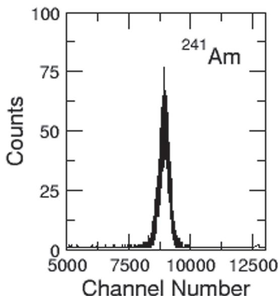
Fig. 4.2.4: Alpha Source -  $^{241}\text{Am}$ , resolution at 5.486 MeV is 4.4%.
