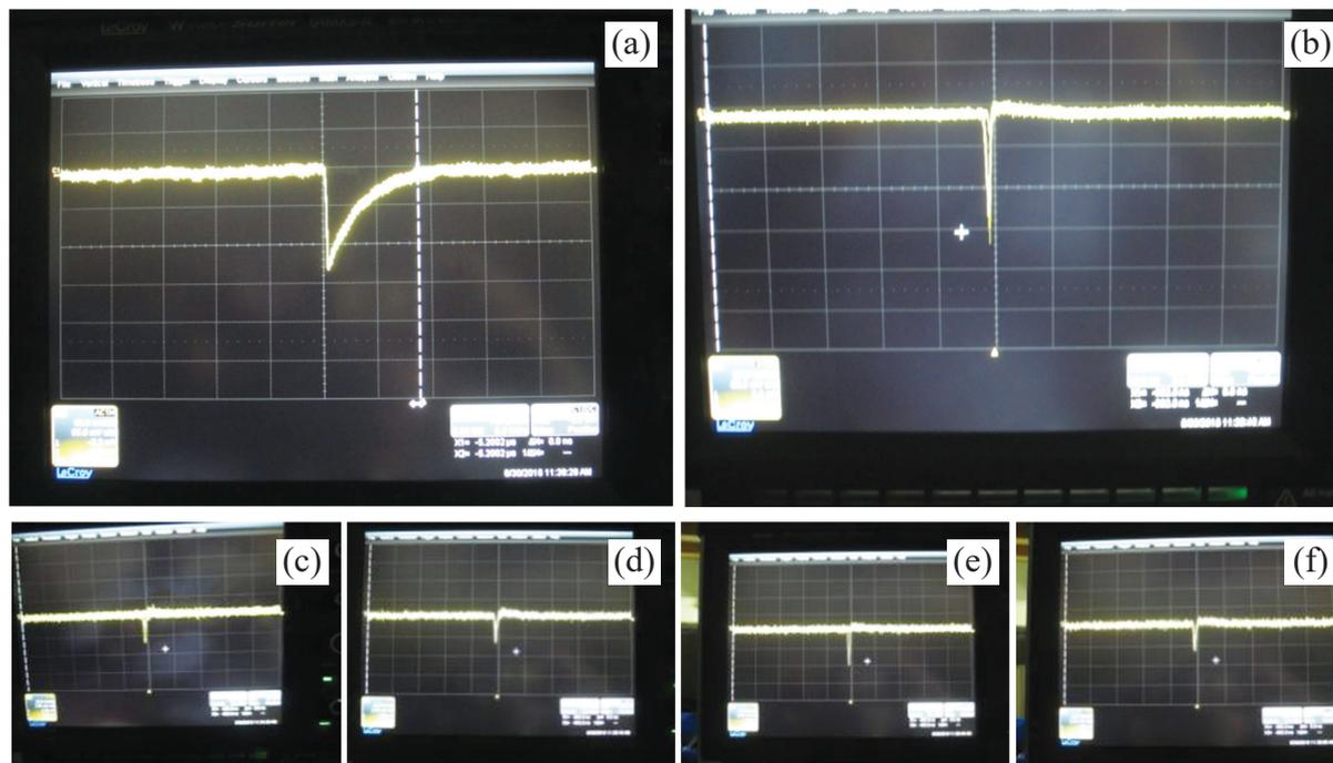
Fig. 4.3.1: Signals from the MWPC, tested with  $\alpha$ -particles from  $^{241}\text{Am}$  – (a) cathode, (b) anode, (c)  $X_{\text{left}}$ , (d)  $X_{\text{right}}$ , (e)  $Y_{\text{up}}$  and (f)  $Y_{\text{down}}$ .
