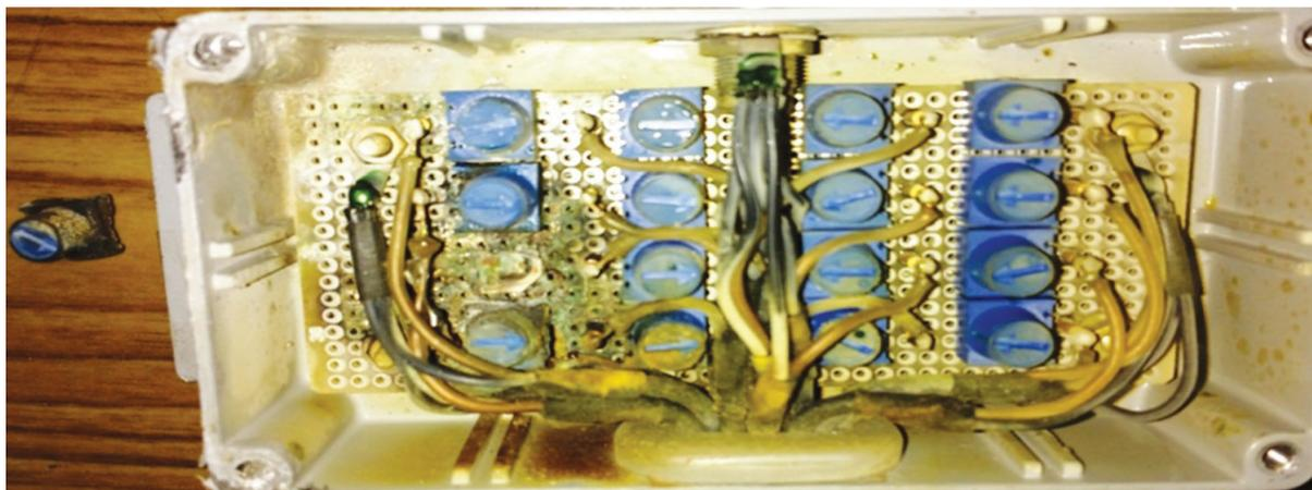
Fig. 4.2.3: ACS high voltage distribution box with damaged variable pot and cables.
