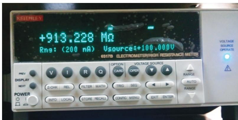
Fig. 4.4.3 Photograph showing standard resistance.
