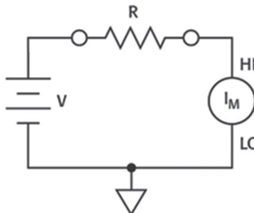
Fig. 4.4.2: The circuit diagram of high resistance measurement set-up.
