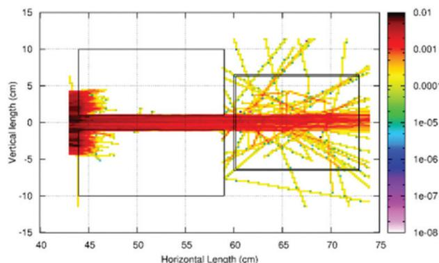
Fig. 4.1.3: Geometrical set-up for FLUKA simulation. The source was positioned 60 cm away from the detector and the beam collimation has been done with thick lead blocks to illuminate the detector selectively. Colour code shows the spatial distribution of gamma ray fluence.
