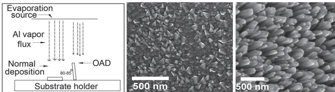
Fig. 4.4.1: (left) Schematic for normal and oblique angle depositions, (centre) SEM image of film grown with normal deposition and (right) SEM image of Al NR formed by OAD.
