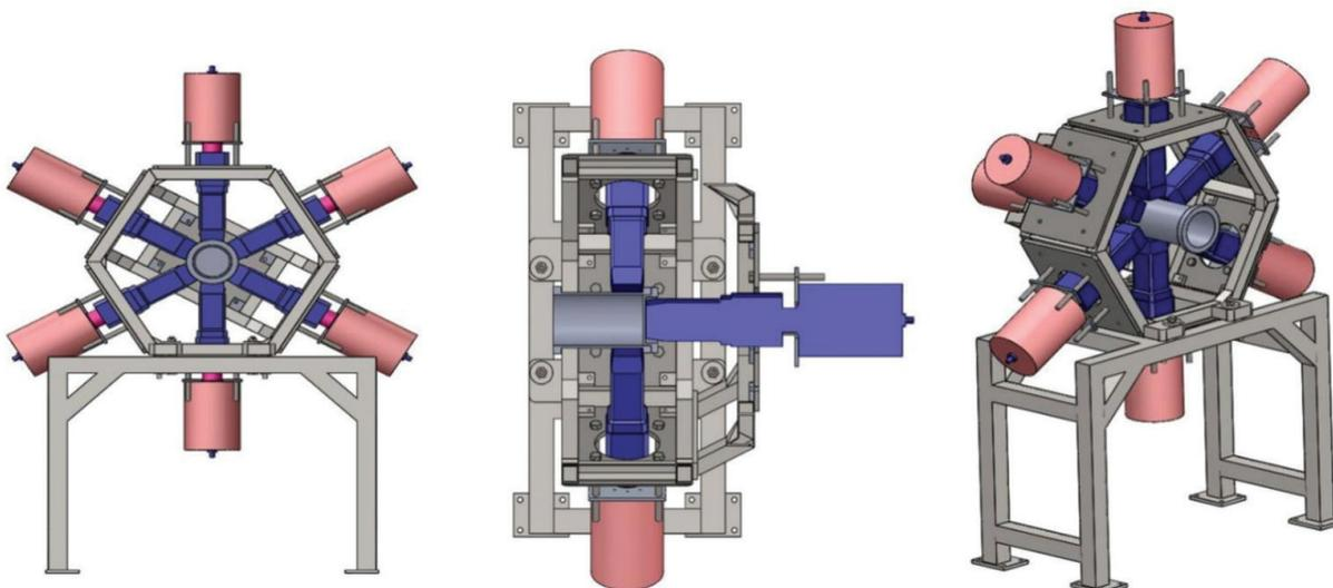
Fig. 4.3.2: Design of dedicated isomer decay setup for HYRA focal plane (cross-sectional and full view).
