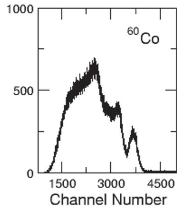
Fig. 4.2.6: Gamma Source- $^{60}\text{Co}$ , resolution at 1.332 MeV is 6.9%.
