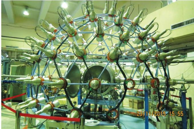
Fig. 4.1.1: The set-up used for measurement of cross-talk in NAND array. Two NaI detectors are mounted close to the source kept inside the chamber.
