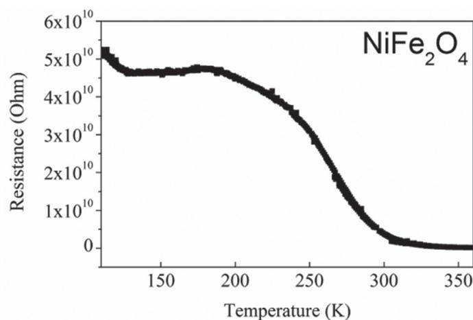
Fig. 4.4.4 Resistance vs Temperature graph for NiFe<sub>2</sub>O<sub>4</sub>.
