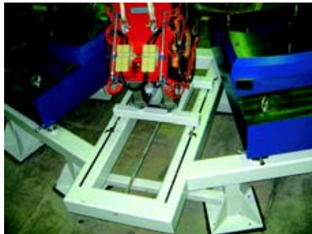
Fig. 6. MD1-Q3-MD2 with alignment pins (final alignment done with top yokes on) and sideways movement mechanism of Q3
