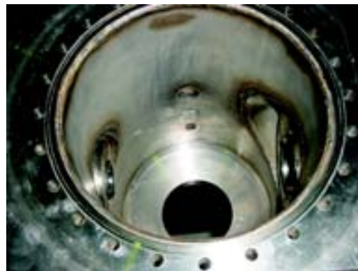
Fig. 8. Inside view - Provision for window foil at entrance and exit side
