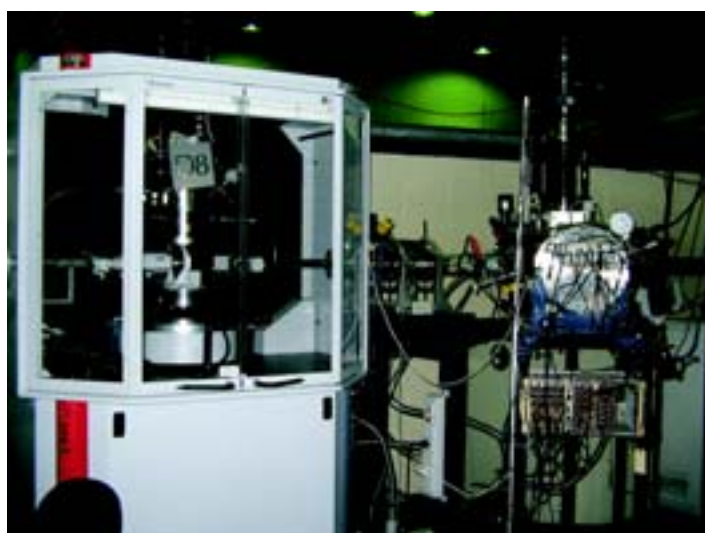
Fig. 2. The beamline in the new beamhall with in-situ XRD set up and LAPSDT detector connected to irradiation chamber.
