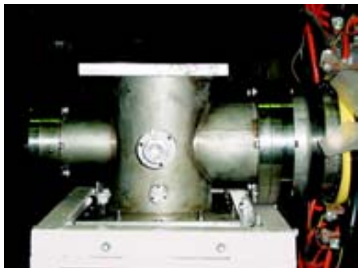
Fig. 7. Target chamber with re-entrant cups for mounting window foil
