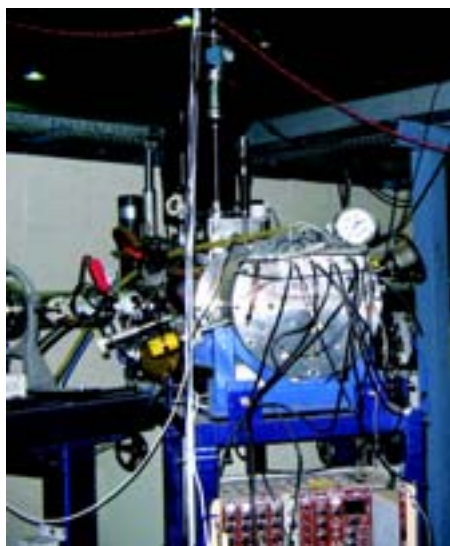
Fig. 1. The irradiation chamber with target ladder mounted on top of Z column and rotational table
