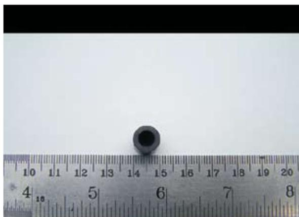
**Fig. 1. Graphite crucible used for evaporation of Pt.**
