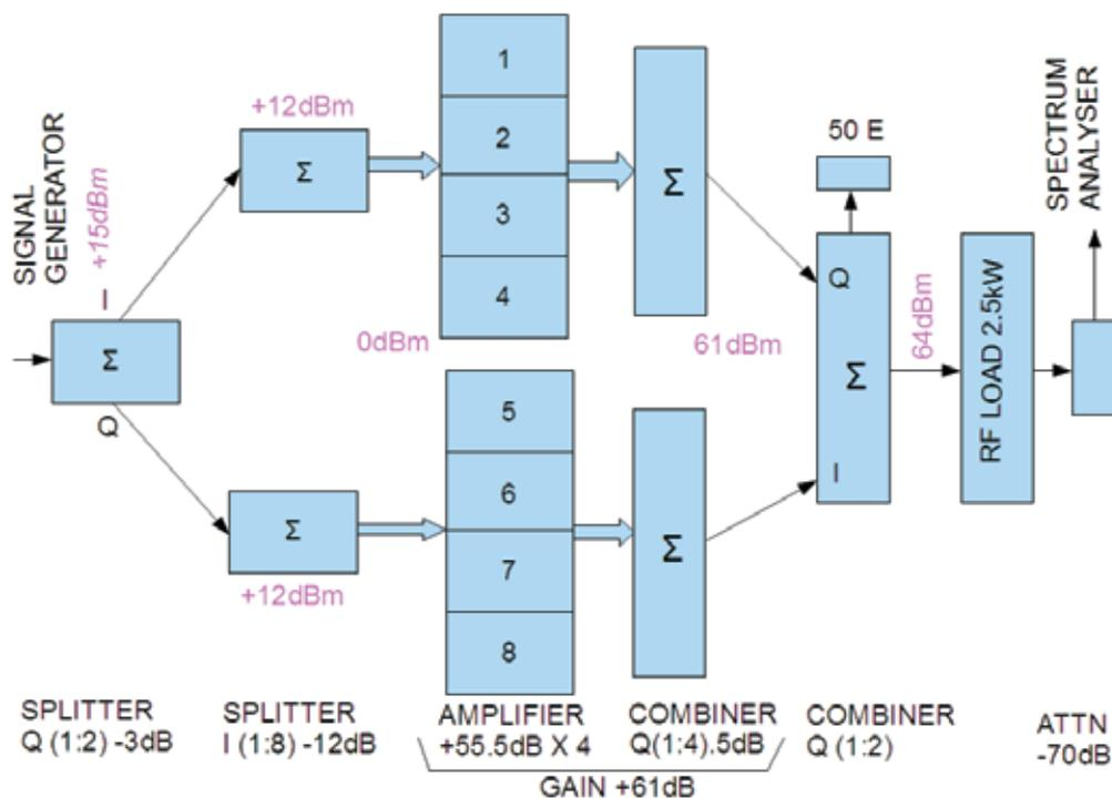
**Fig. 1. Schematic diagram of 2kW solid state power amplifier**
