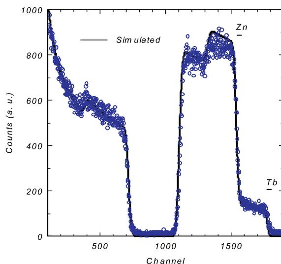
**Fig. 2. RBS spectrum of ZnO-Tb co-sputtered thin film.**
