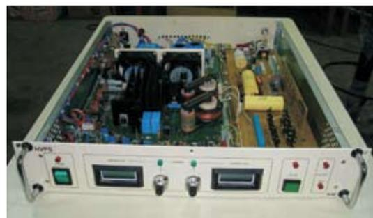
**Fig. 3. High Voltage Power Supply**
