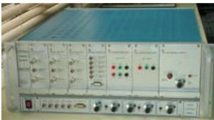
Fig. 4. Three channel Linear high voltage ( $\pm 2\text{kV}$ ) amplifier
