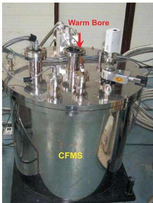
**Fig. 8. Warm bore Cryogen-free superconducting magnet system**
