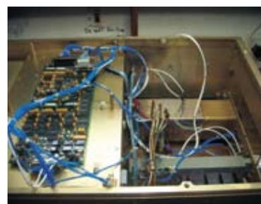
(C) TWTA with modules open for tube replacement
