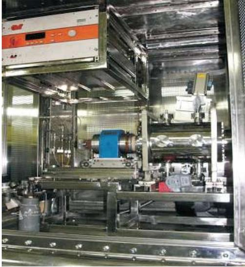
**Fig. 5. Source on High Voltage Plat form**
