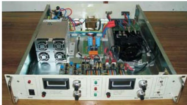
**Fig. 5. TEC based rapid thermal cycler**
