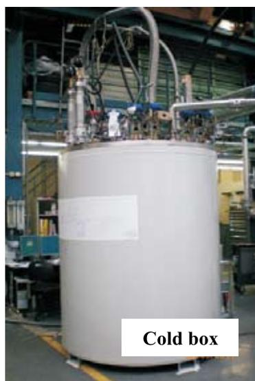
**Fig. 3. Picture of the Cold Box of 750 W Helium refrigerator**
