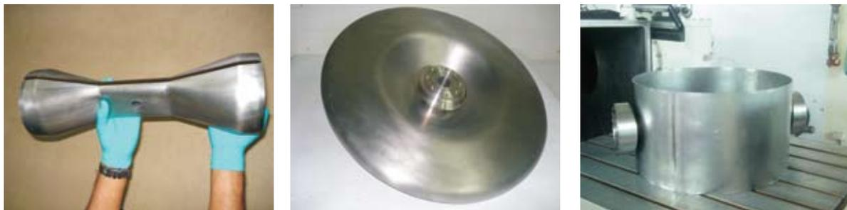
**Fig. 6. Welded niobium Spoke (left), End Wall with the Beam Port (center), Outer Shell with Coupler Port flanges (right)**
