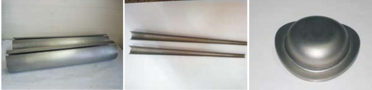
**Fig. 5. Niobium components for the prototype low beta resonators – Outer Housings (left), Central Conductor halves (center), and saddle shaped Cup for the Beam Port on the Outer Housing (right)**
