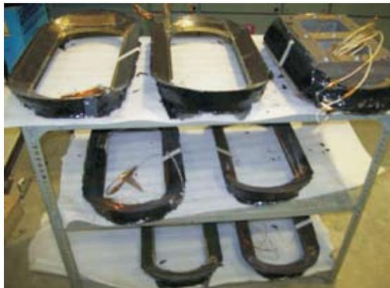
**Fig. 10. HYRA Quadrupole magnet coils**
