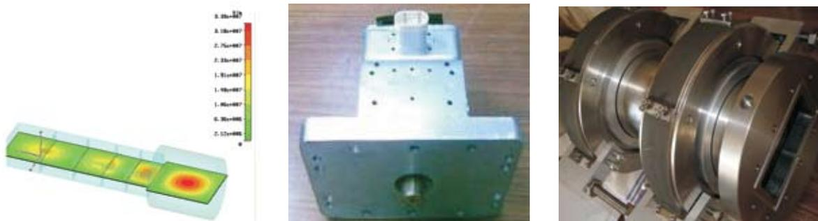
**Fig. 12. 4 step quarter wave transformer coupled to the ECR cavity showing the  $\text{TE}_{111}$  mode; (Right) Magnetron and part of the assembled 2.45 GHz ECR source**
