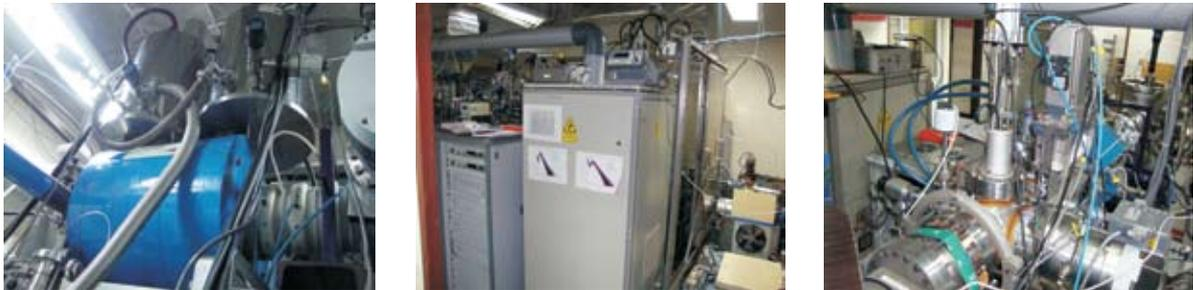
**Fig. 1. (Left)A view of the 18 GHz HTS ECR-PKDELIS; (Middle) 18 GHz RF generator, HTS instrumentation electronics, cooling systems; (Right) post-analyser section**
