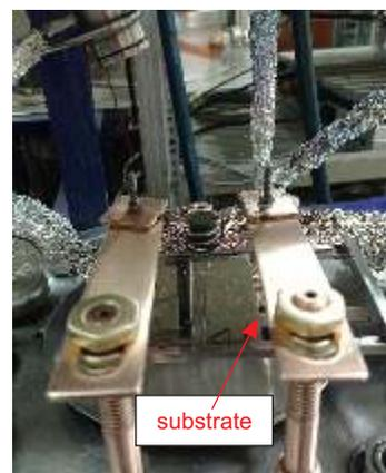
Figure.2: Inverted evaporation source.
