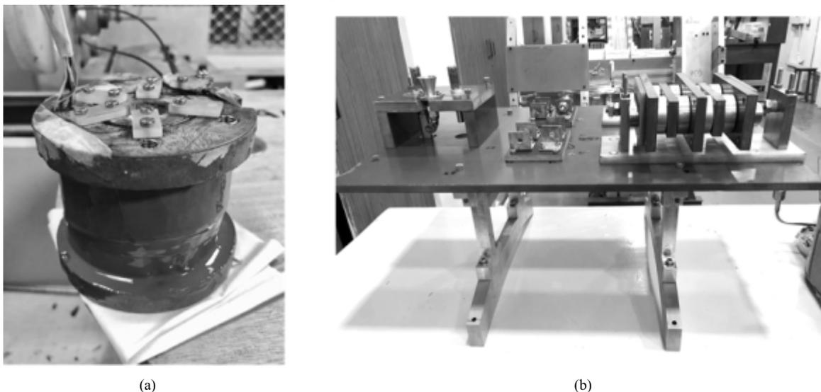
Fig 3.1.2.7 (a) The superconducting switch of the MRI magnet, and (b) one of the ancillary boards equipped with few ancillaries.
