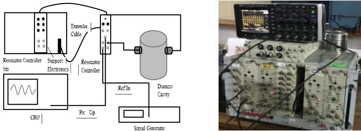
Fig. 3 Block Diagram and Test Setup of LLRF Controllers of Linac
