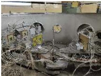
Fig.3: Detector system for multi-nucleon transfer measurements below Coulomb barrier.
