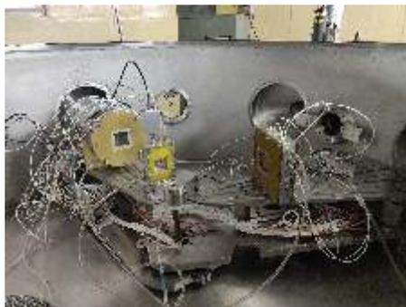
Fig.1: Detector system for multi-nucleon transfer measurements above Coulomb barrier.
