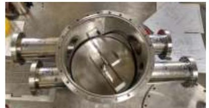
Electrostatic Analyzer Vacuum Chamber
