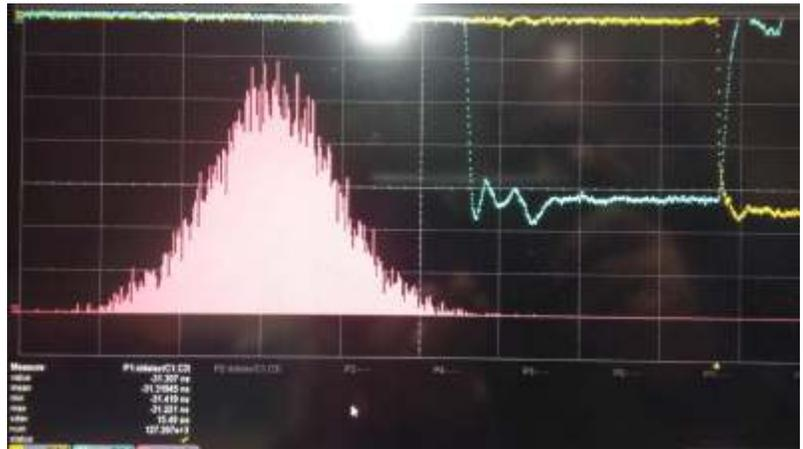
Fig 2 Delay and jitter of busy logic
