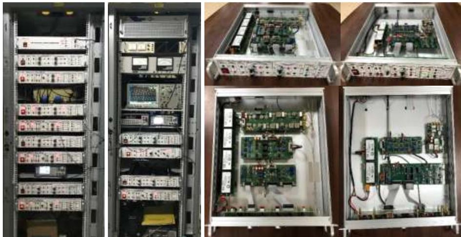
Fig. 4 LLRF Controls Racks and Inner view of Electronics
