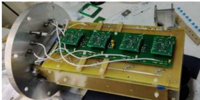
Fig.2: Split anode ionization chamber with integrated CSPA units for signal processing.
