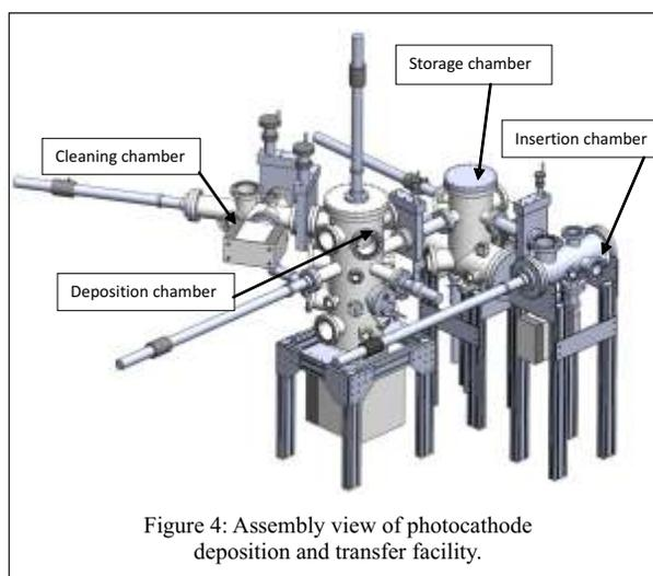
Figure 4: Assembly view of photocathode deposition and transfer facility.
