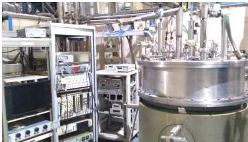
Fig. 3.1.2.2 Simple test cryostat at IUAC.
