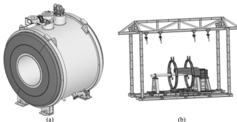
Fig 3.1.2.6 (a) The zero-boil-off MRI cryostat, and (b) the magnet-cryostat assembly jigs and fixture.
