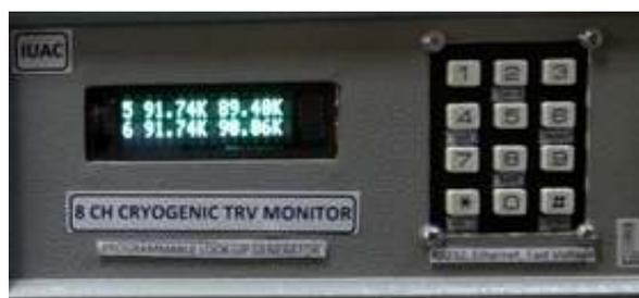
Fig. 3: A Prototype TRV Device
