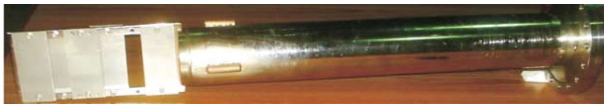
Fig. 9. Fixed slit system, used at Q3 centre in momentum achromat (vacuum) mode, for secondary RIB selection
