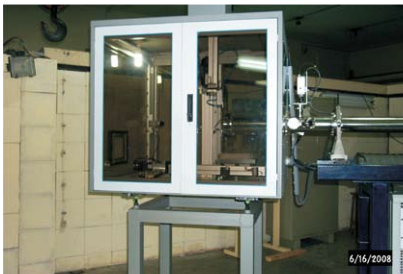
Fig.1. Multi axis positioning system Aspire in the beam line
