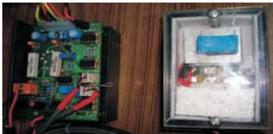
Fig. 10A. Temperature pulse generator
