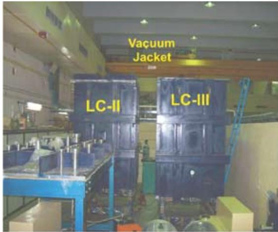
**Fig. 4. Vacuum Jackets of 2nd and 3rd Linac Module**
