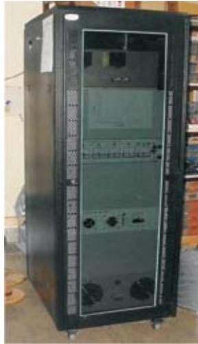
**Fig. 11. Tube based 2kW RF amplifier**
