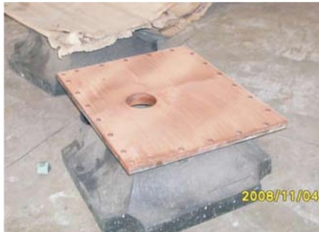
**Fig.1. Copper electroplating of side plate of RFQ chamber**
