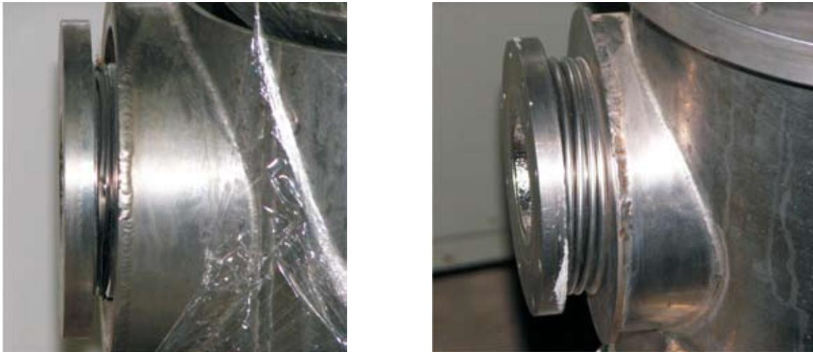
**Fig.2. Transition flanges with SS-Edge welded bellows (shown in left) are now replaced with the transition flanges with SS-formed bellows (shown in right)**
