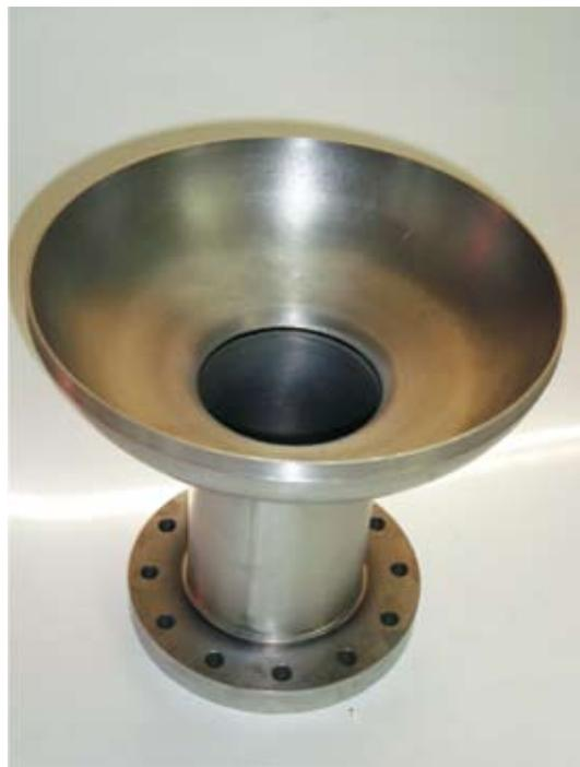
**Fig. 8. Niobium Half Cell of the Tesla-type Single Cell Cavity.**
