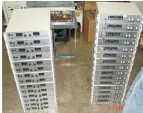
**Fig. 9. Super conducting magnet power supply and Programmer**
