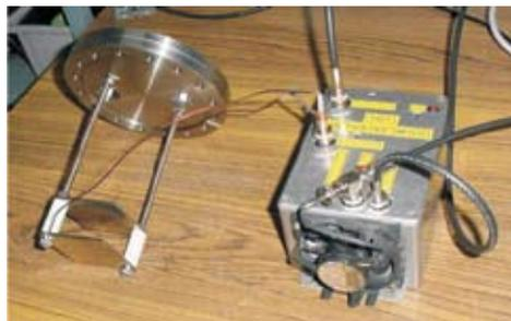
**Fig. 12. Fast high voltage switch**
