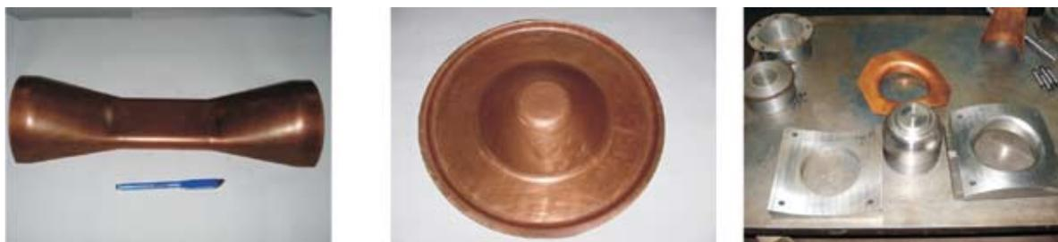
**Fig. 6. Half Spoke (left), End Wall (center) and Spoke to Shell Collar (right) formed in copper. The forming die for the Spoke to Shell Collar can also be seen in the foreground of the picture on the right.**
