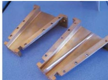
**Fig. 11. View of the 2.45 GHz, 2 kW RF injection line (left) and quarter wave transformer (right)**
