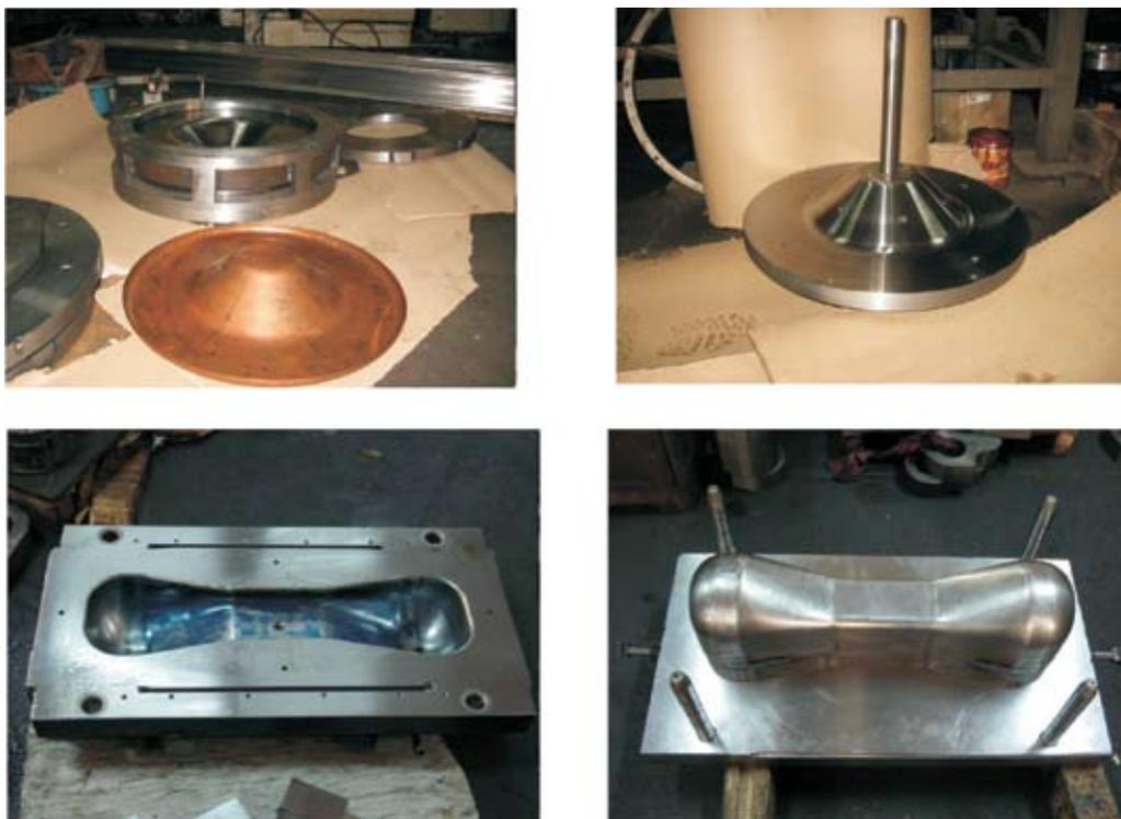
**Fig. 5. Dies for forming the End Wall (above) and the Half Spoke (below).**
