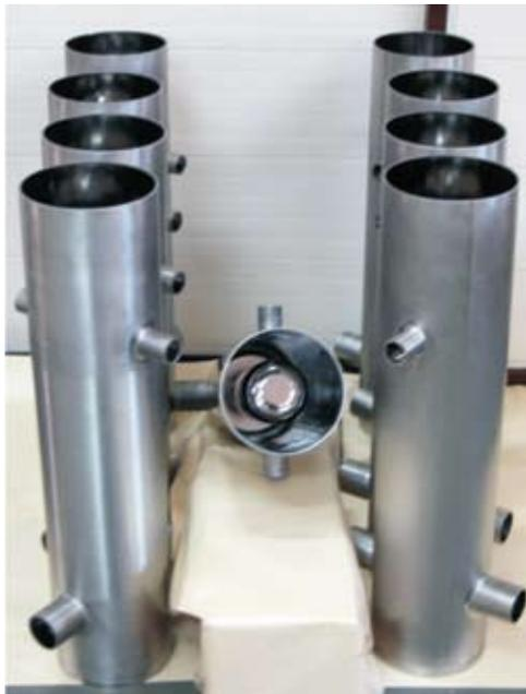
**Fig. 1. Bare niobium Quarter Wave Resonators**
