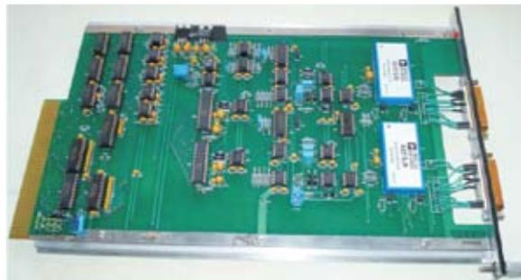
**Fig. 7. CAMAC based controller for scanning magnet power supply**
