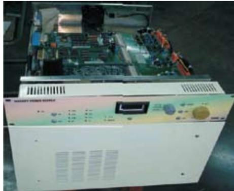
**Fig. 6. HCI magnet power supply**
