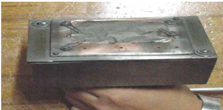
**Fig. 3. Copper mounted on substrate heater**
