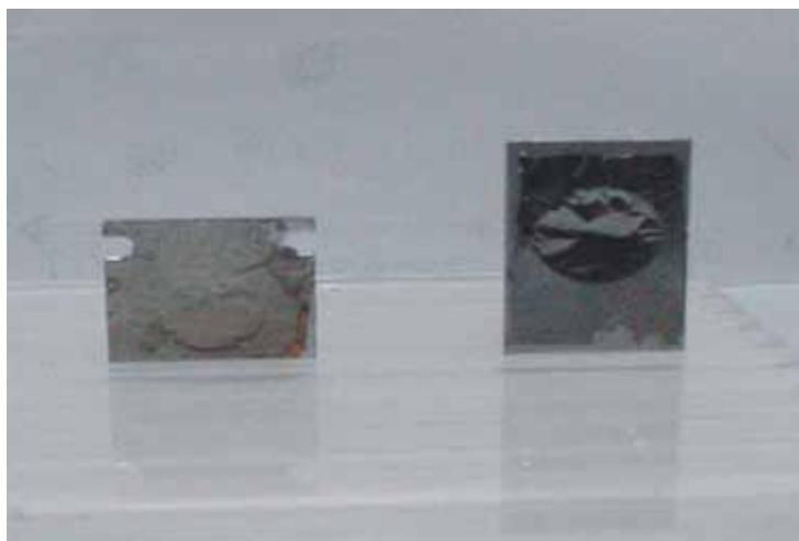
**Fig. 4. Tantalum target on carbon backing (right) and self supporting (left).**
