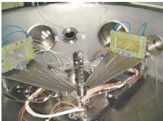
**Fig.9B. MWPCs mounted in GPSC**
