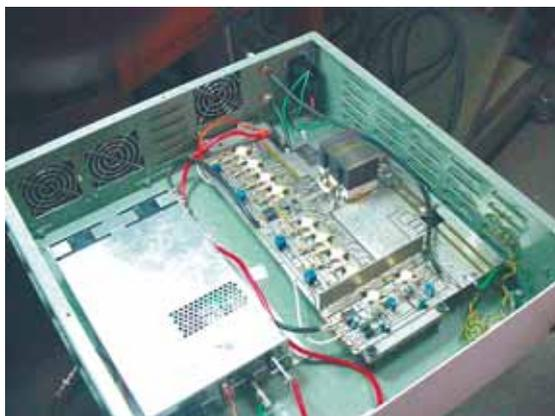
**Fig. 3. Inside view of 12MHz RF power amplifier**
