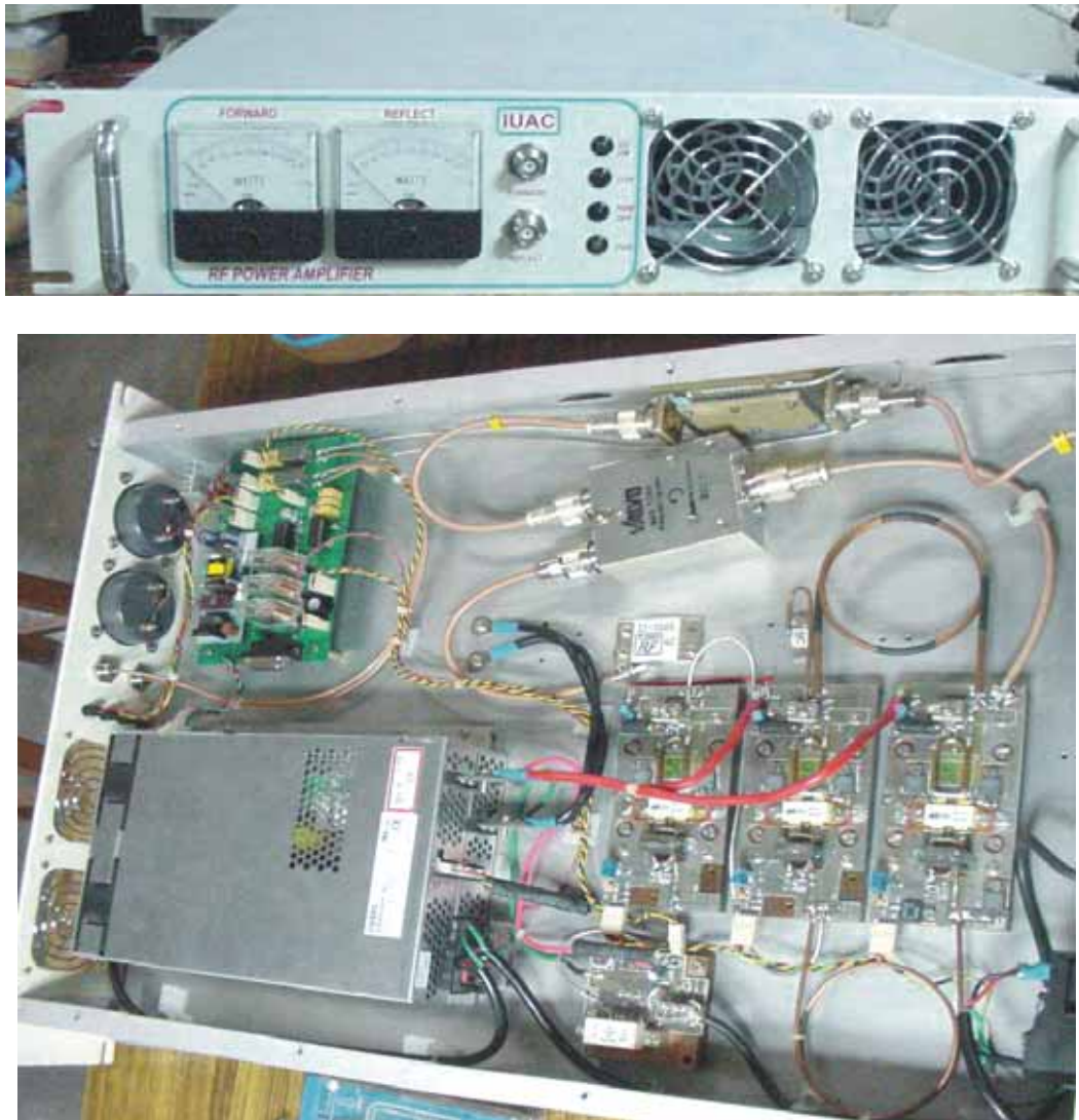
Fig. 1. 400Watts VHF Power amplifier
