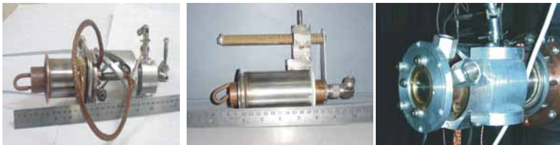
Fig. 1. Three different drive couplers were fabricated and tested to solve the problem of the old drive couplers
