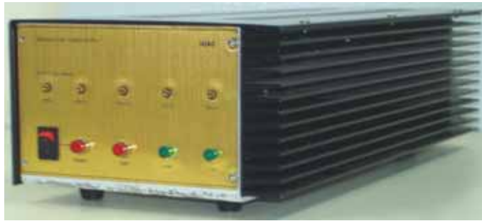
Fig. 9 : Pre-amplifier Power Supply
