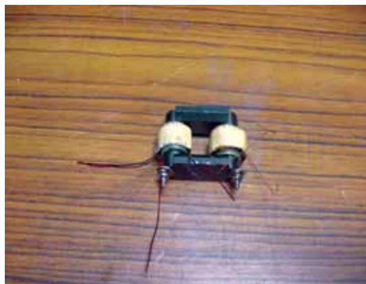
Fig. 4. View of the high frequency transformer
