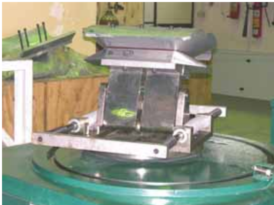
Fig. 10A. Flipping mechanism of winding machine
