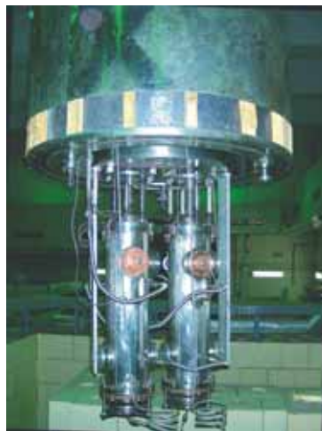
Fig. 4. Figure shows two QWRs loaded in the rebuncher cryostat prior to their first offline cold test
