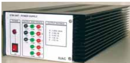
Fig. 11. STM Unit Power Supply
