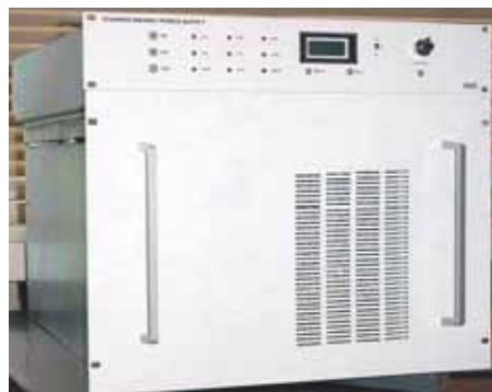
Fig. 7. High Current Scanner Magnet Power Supply
