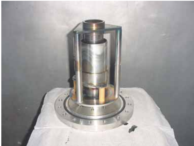
Fig. 2. View of the Einzel lens after it was found shorted
