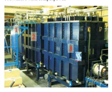
Fig. 2. The remaining cryostats 2 and 3 installed in the beam line
