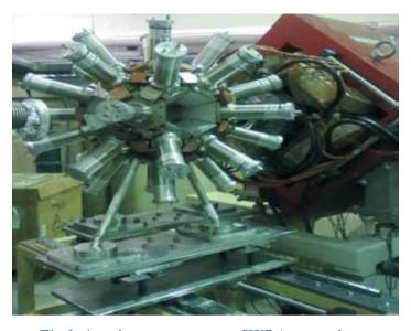
Fig.1.  $4\pi$  spin spectrometer at HYRA target site on specially made structure
