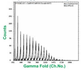
Fig. 4. Gamma fold spectrum (ER gated) superimposed with scaled down (7.5%) singles gamma fold; Lower fold contamination is removed by ER gating; Matching of higher folds indicate ER transmission efficiency of 7.5%
